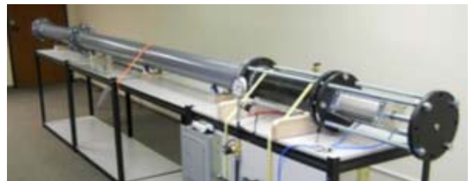
FIGURE 1. 6-IN INTERNAL DIAMETER SHOCK TUBE USED TO GENERATE FRIEDLANDER SHAPED BLAST WAVES.
