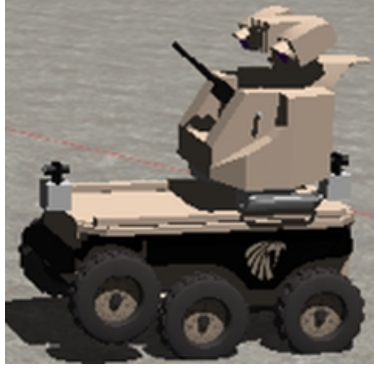
Figure 11: The demonstration vehicle, Landshark, with four rotation degrees of freedom. The camera rotates on the vertical and horizontal axes. The turret rotates around the vertical axis, and the paintball gun rotates around the horizontal axis.
