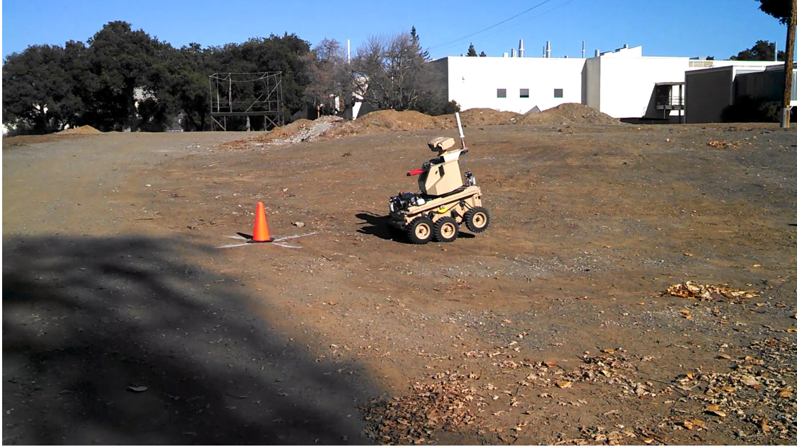
Figure 13: Scene from the live demonstration of actual code generated by the integrated approach. Using a SPIRAL generated implementations of a KeYmaera X proven monitor, and sensor fusion to guard against GPS spoofing, the Landshark robot stopped safely in front of an obstacle.
