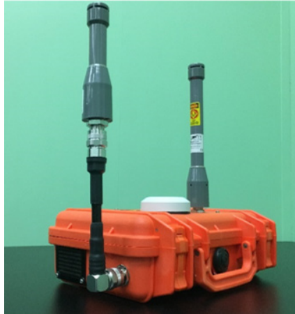
Fig. 3 Node exterior depicting the SDSS assembly including the GPS puck antenna, 2.4-GHz MANET antenna, and 5.8-GHz SDR antenna
