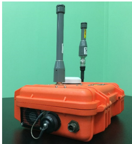
Fig. 4 Node exterior depicting the 2-pin power connector and auxiliary Ethernet port
