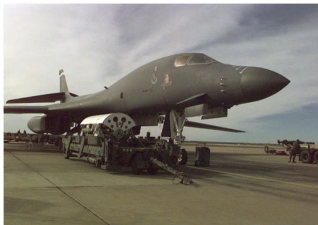
Figure 1. 2 B-1 Rotary Launcher on an MHU-196 Trailer
