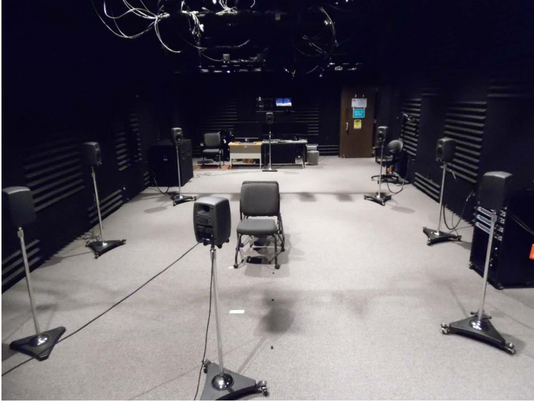
Fig. 5 ARL-HRED indoor EAR facility used to measure speech intelligibility performance
