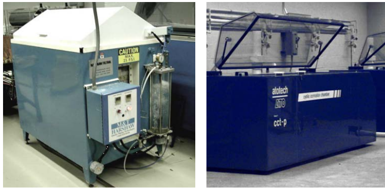
Fig. 6 The chamber used to conduct the neutral salt fog ASTM B117 (left) and the chamber used to conduct GM9540P tests (right)
