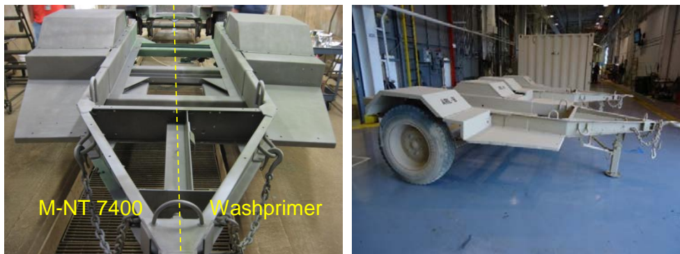
Fig. 52 M200A1 trailer with split pretreatments (left) and with full CARC system (right)
