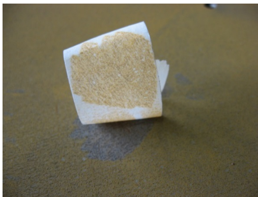
Fig. 57 Result of masking tape pull on dried PPG 11-TGL-27 treated assets
