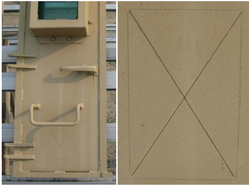
Fig. 49 MRAP door with Oxsilan 9810/2 after 2 years with close-up of scribed area
