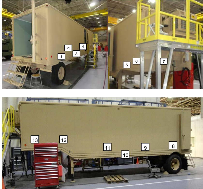
Fig. 63 The M373A2 trailer pretreated with baseline DOD-P-15328 wash primer and complete CARC system. The numbers indicate where adhesion tests were performed.
