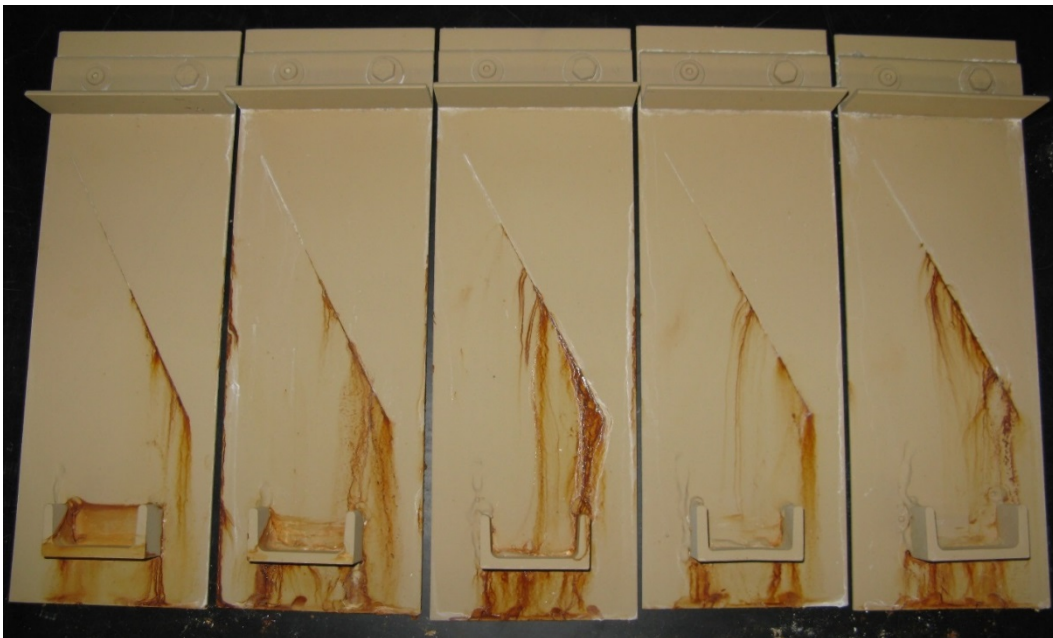
Fig. 19 DOD-P-15328 on multimetal panels with MIL-DTL-53022 after 1008 h
