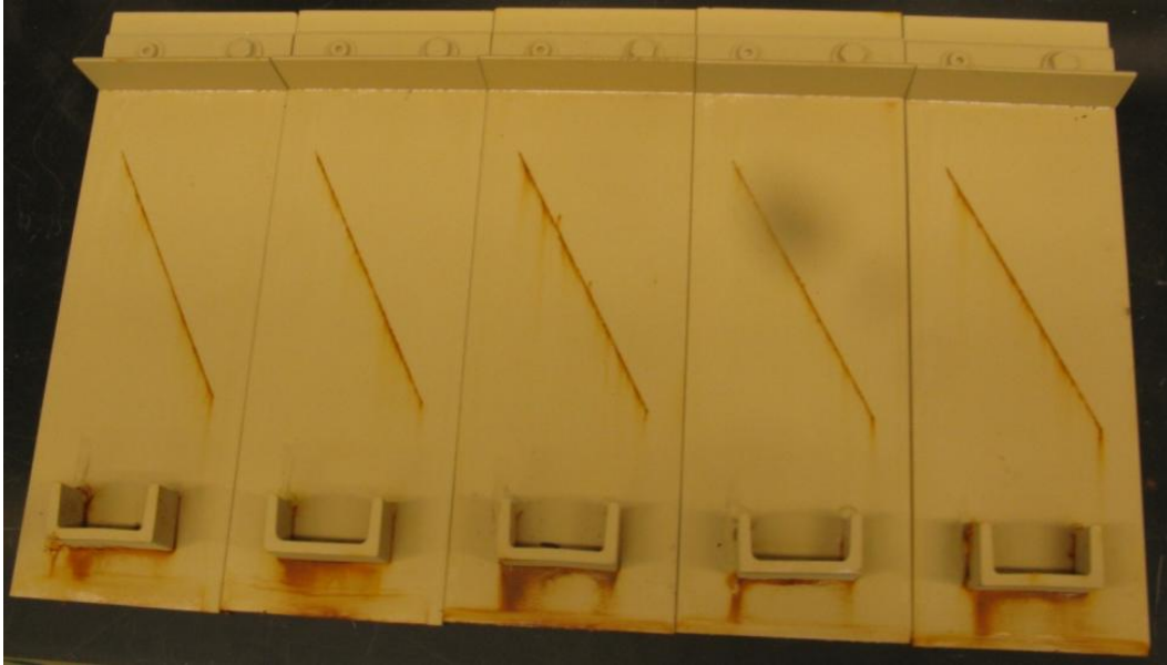
Fig. 34 Bonderite M-NT-7400 on multimetal panels primed with MIL-DTL-53030 after 80 cycles
