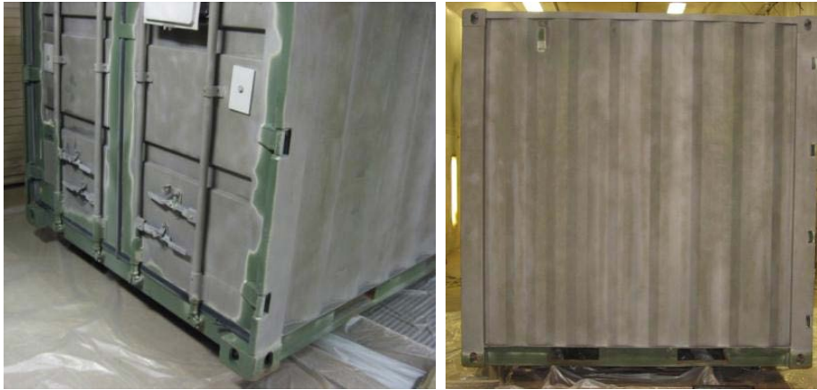
Fig. 51 Abrasive blasted tricon before (left) and after (right) Bonderite M-NT 7400
