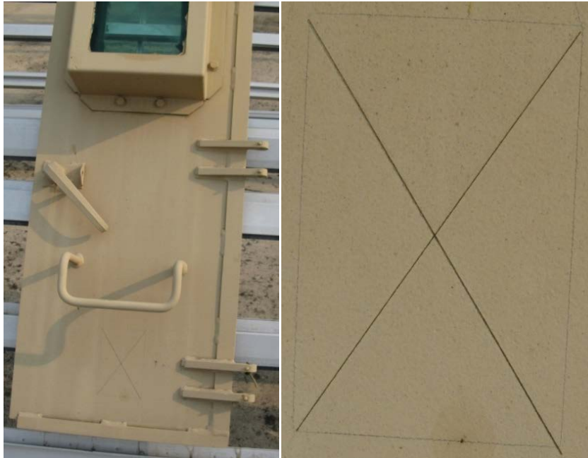
Fig. 50 MRAP door with DOD-P-15328 WP after 2 years with close-up of scribed area
