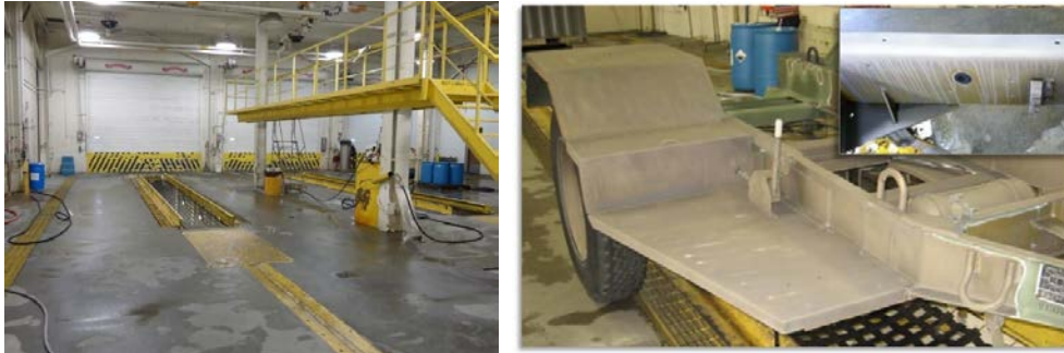
Fig. 53 Wash bay at LEAD (left) and M200A1 trailer (right) treated with Oxsilan 9810/2 showing what appears to be slight flash rust in some areas
