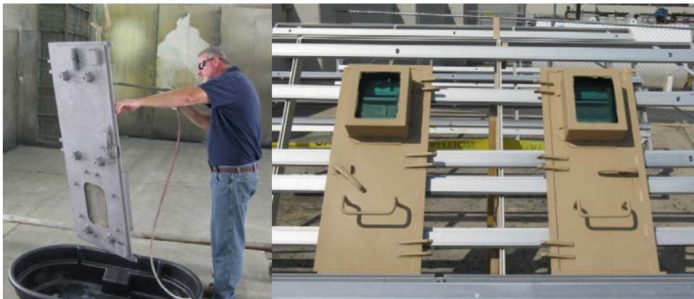
Fig. 48 MRAP door being treated with Oxsilan 9810/2 (left); painted doors on outdoor exposure racks at ARL (right)
