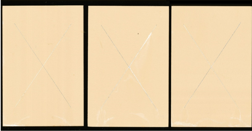
Fig. 15 Bonderite M-NT-7400 rated a 9 on Al panels with MIL-DTL-53030 at 1000 h
