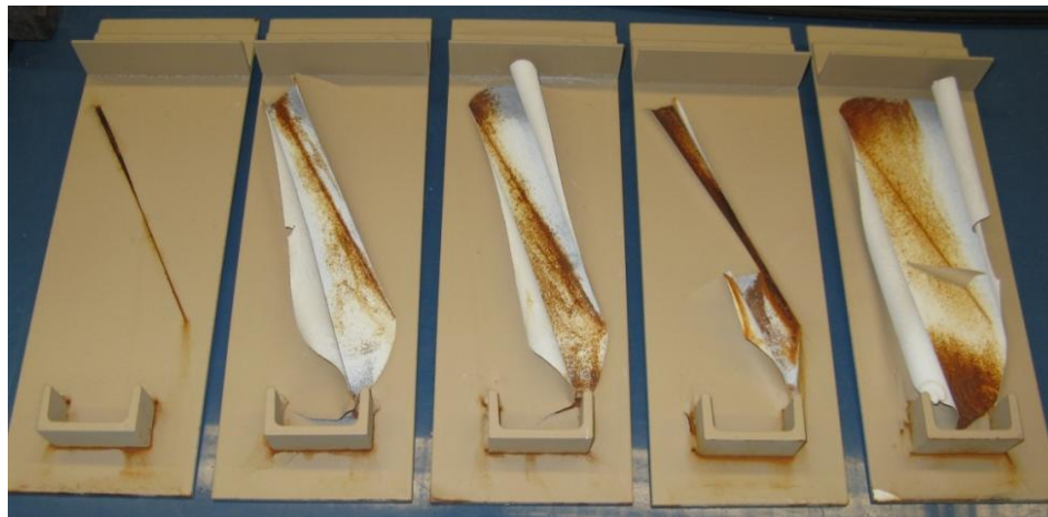
Fig. 32 NCP nonchromate wash primer multimetal panels delaminating after 3 cycles
