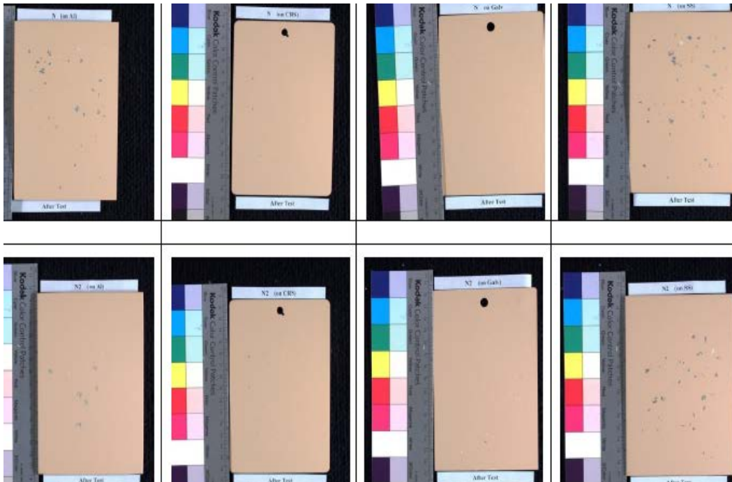
Fig. 11 DOD-P-15328 wash primer on (from L to R) aluminum, cold-rolled, galvanized, and stainless steel (53030 top, 53022 bottom)
