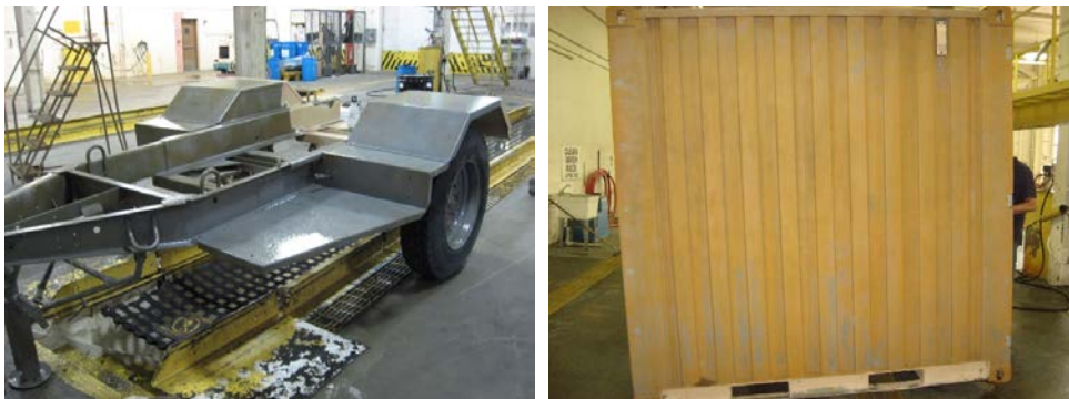
Fig. 56 M200A1 trailer during treatment (left) and container dry following treatment (right) with PPG 11-TGL-27
