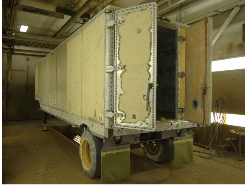
Fig. 62 Prepped M373A2 trailer ready for pretreatment application
