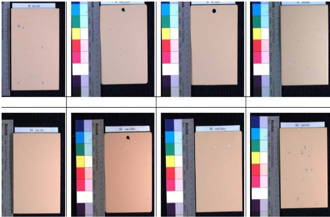
Fig. 9 Bonderite M-NT-7400 on (from L to R) aluminum, cold-rolled, galvanized, and stainless steel (53030 top, 53022 bottom)
