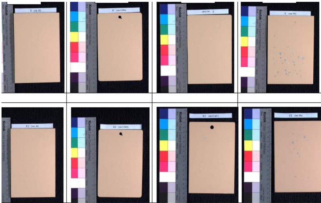
Fig. 10 Ecosil 5-1 on (from L to R) aluminum, cold-rolled, galvanized, and stainless steel (53030 top, 53022 bottom)
