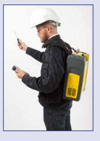
A unique part of the Model DX4040 is Gasmet Technologies GICCOR (an acronym for 'Genzel interferometer with a cube corner retroflector') interferometer. The interferometer can be thought of as the engine of a FTIR. It is rugged and withstands the demanding environmental conditions of nonlaboratory environments.
