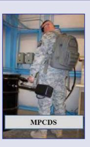
this instrument. When nuclear material is detected, an attachment can be quickly connected to enable the fast determination of isotopic enrichment of the material. This rugged instrument is currently at the TRL-6 level, and has undergone extensive testing.
