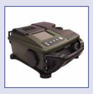
GUARDION is ready to operate within five minutes from a cold start. The CUSTODION™, a solid phase microextraction (SPME) fiber syringe, is used for simple sample collection and injection into the GC/MS system.
