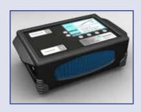
the user introduces a swab of unknown material into the system, the unit will automatically perform the steps of sample recovery, lysing, purification, realtime PCR amplification, and fluorescence detection in order to determine if the material contains genetic material with a sequence matching an on-board library of known threats.
