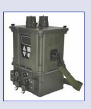
health (IDLH) levels. It also provides chemical details including class, type, concentration and dosage as well as CWA identification.
