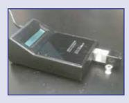
rapid, point-of-care bacteria detection system that only detects live bacteria. The test system is portable and can be taken into the field for monitoring of bacteria and easily used by non-laboratory personnel. Test time is under one minute. Detection limits go down to 100 CFU. The product is commercial and currently is used for bacteria detection in healthcare, food and water applications.
