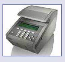
$(\pm 0.25$ °C from 35°C to 100°C) and long term stability and high reliability. The sample block accommodates several different types of MicroAmp® disposable tubes and plates, which must be used in order to create a sealed chamber.
