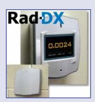
they are in range of a single Rad-DX system (up to 1000 meters)! The Rad-DX units will automatically form an intelligent, self-healing mesh network, allowing them to be constantly connected to each other as well as to the user network.
