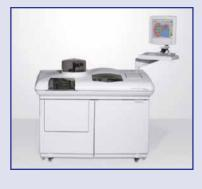
of usable walk away time Third-generation assays for excellent sensitivity Comprehensive menu of more than 100\* assays Easily automate through VersaCell™ or other ADVIA Automation Systems The IMMULITE 2000 analyzer combines allergy and specialty immunoassay testing on one platform with many features that provide greater efficiency in the lab. The IMMULITE sample types include serum, plasma, urine, and amniotic fluid but are assay specific.
