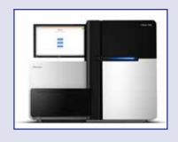
Cluster Generation System, a suite of data collection and analysis software, and dedicated consumables. cBot provides automated clonal amplification of single molecules randomly distributed on a glass surface. Resulting DNA clusters are sequenced on the HiSeq 2000 using sequencing by synthesis method with patented reversible terminator chemistry.
