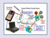
Jyophilized intrachain or competitive FRET-aptamer reagents with long shelflives in capped plastic cuvettes. The handheld fluorometer OEM is Turner Biosystems or Promega and OpTech produces the patented FRET-aptamer reagents (US Patent No. 7,906,280).
