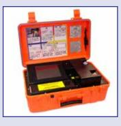
the chemical sampling interface. The sampling interface consists of two ports (inlet and exhaust) leading to the 44 cm path length transmission cell and accommodates either of two sample collection devices provided with the system. Because the GasID has exposed ports, the instrument is not recommended for use in the hot zone, rather, the sample collection devices are decon-able and permitted for use in the contaminated area of interest.
