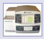
buccal swab samples and sample processing is initiated with no further user interaction. The system extracts DNA from the samples and performs STR amplification, electrophoretic separation and software analysis to generate full DNA profiles in about 90 minutes. For the U.S. market, the results data are saved in CODIS-compatible format within the embedded GeneMarker HID® software (SoftGenetics®, LLC). Other data formats will be available as needed.
