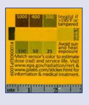
RADSticker monitors 50–10,000 mSv. When exposed to ionizing radiation, the sensor of the dosimeter develops blue color instantly and the color intensifies as the dose increases. Radiation exposure can be estimated simply by matching the colors of the sensor with the adjacent color reference bars. If used as per instruction, RADSticker will not give false signals. The operating temperature range is from -30oC to 90oC. All essential information is privided in one page manual.
