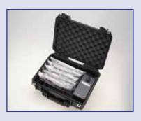
ricin and botulinum toxins. In less than 15 minutes reliable information is obtained, allowing the First Response team to make an informed decision regarding incident closure. The Microbe Screen™ is performed using a proven fluorescent-based technology in a hand-held reader and the Toxin Screen™ is carried out using lateral flow antibody tests.
