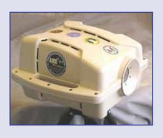
rapid data acquisition capability needed to operate from moving platforms without degradation of sensitivity. The system's real-time processor provides immediate identification, display, and geo-location of threats using integrated GPS and pointing systems. On board capability is present to transmit threat location via the Joint Warning and Reporting Network.
