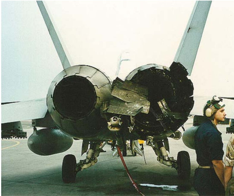
Figure 7 USMC F/A-18D with damaged turkey feathers after being hit by a MANPAD during Operation Desert Shield. Reprinted from http://armyphotos.net/
