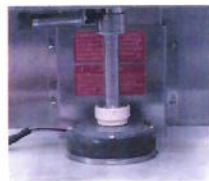
Figure 4: Gel sample on the SR5 Rheometer
