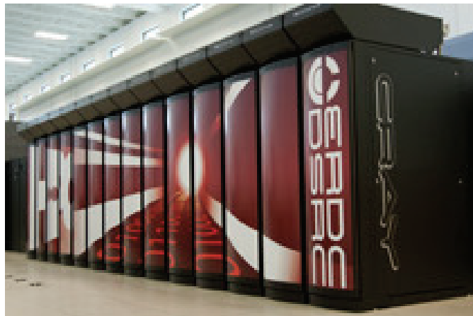
Figure 15. Garnet. Cray XE6 - 1.5 PFLOPS (Courtesy of ERDC-HPC-DSRC).
