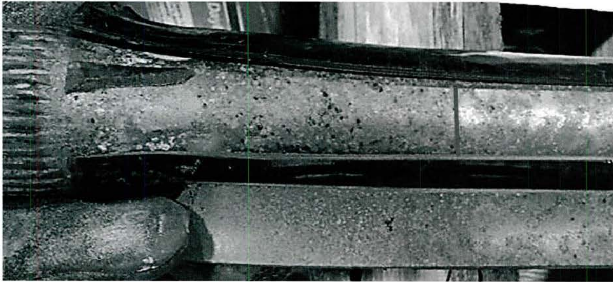
Figure 63 - Corrosion under Disbonded Coating on Torsion Bar
