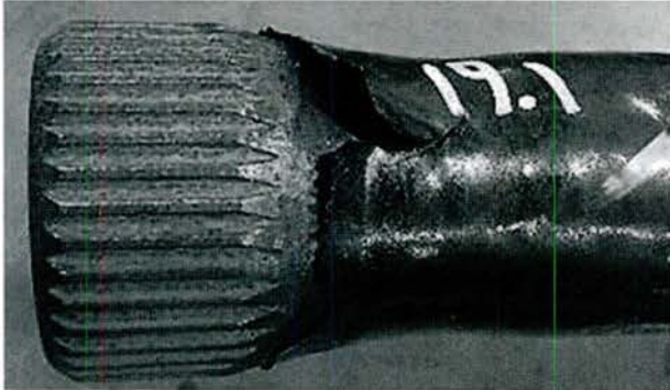
Figure 35 - Coating Edge Damage on a Torsion Bar
