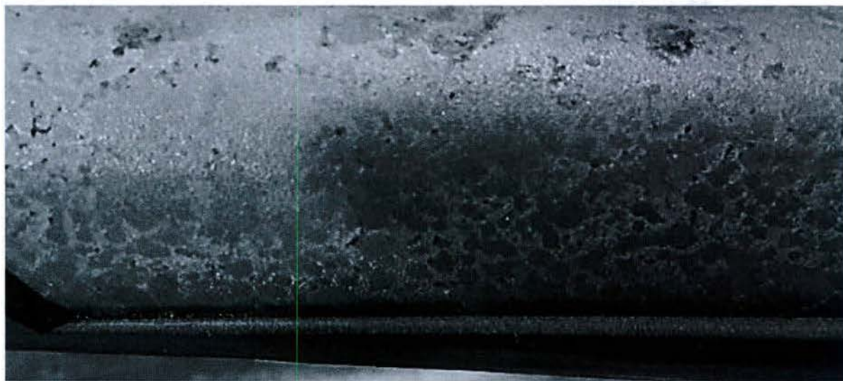
Figure 66 - No Corrosion Observed Under Polyethylene Coating with Good Adherence
