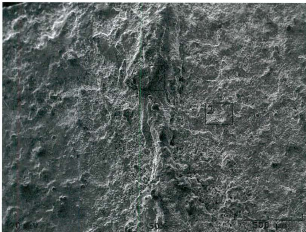
Figure 23 - SEM Photomicrograph of Heavy Corrosion Region in Specimen 15 (Mag 50x)
