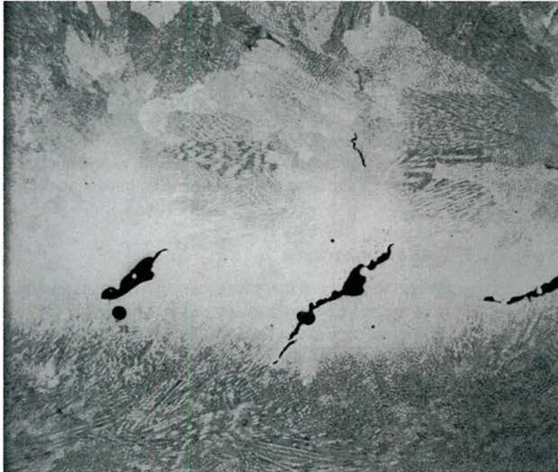
Figure 54: 50x Photo showing interlayer voids
