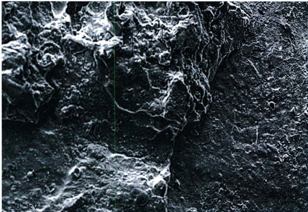
Figure 55 - SEM Photomicrograph of the Thick (left) and Thin (Right) Corrosion Layers on Torsion Bar 55-2
