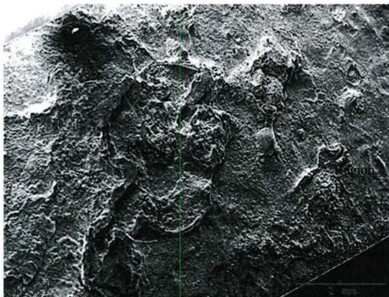
Figure 53 - SEM Photomicrograph of the Corrosion on Torsion Bar 55-2
