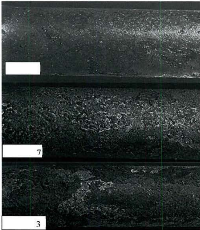
Figure 169 - Optical Photomicrographs of Tensile Specimens after Chemical Cleaning (Mag 10x)
