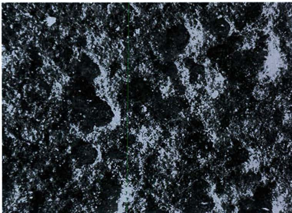
Figure 13 - Optical Photomicrograph of Surface of Specimen 12D (Mag 20x)
