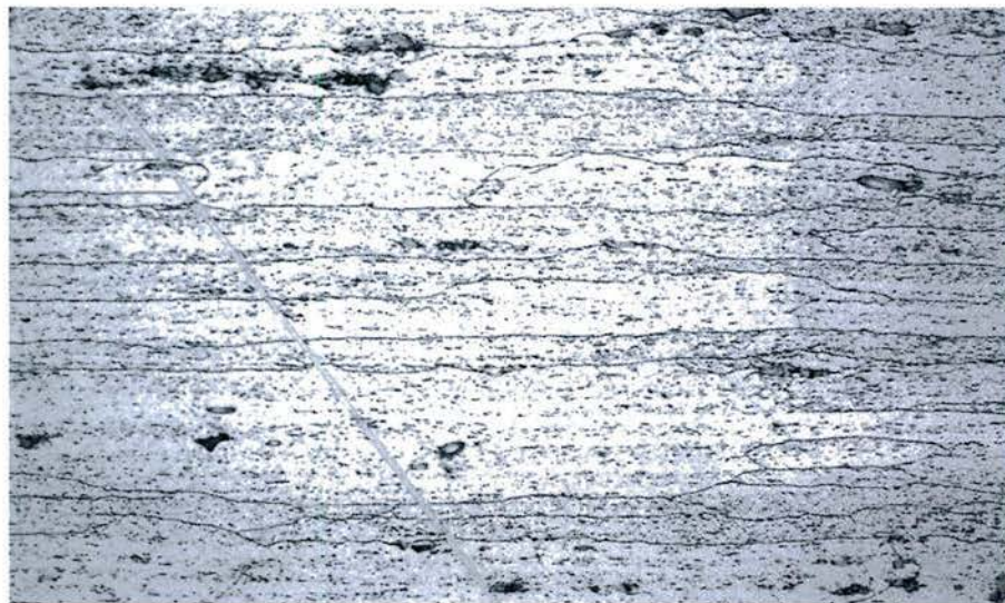
Figure 16 - Optical Photomicrograph -5083 Microstructure, Region 2 after 40% Phosphoric Acid Etch (Mag 500x)
