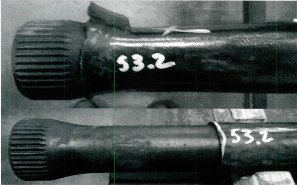
Figure 46 - Torsion Bar 53-2 Scrapped for Coating Disbonding. Top View Shows Coating Disbonding, Bottom View Shows Torsion Bar Surface after Coating Removal
