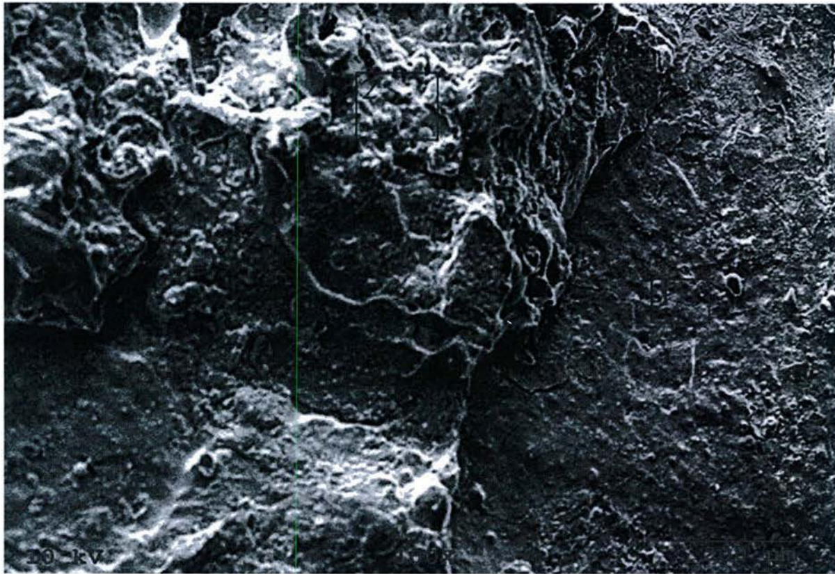
Figure 45 - SEM Photomicrograph of the Thick (left) and Thin (Right) Corrosion Layers on Torsion Bar 55-2
