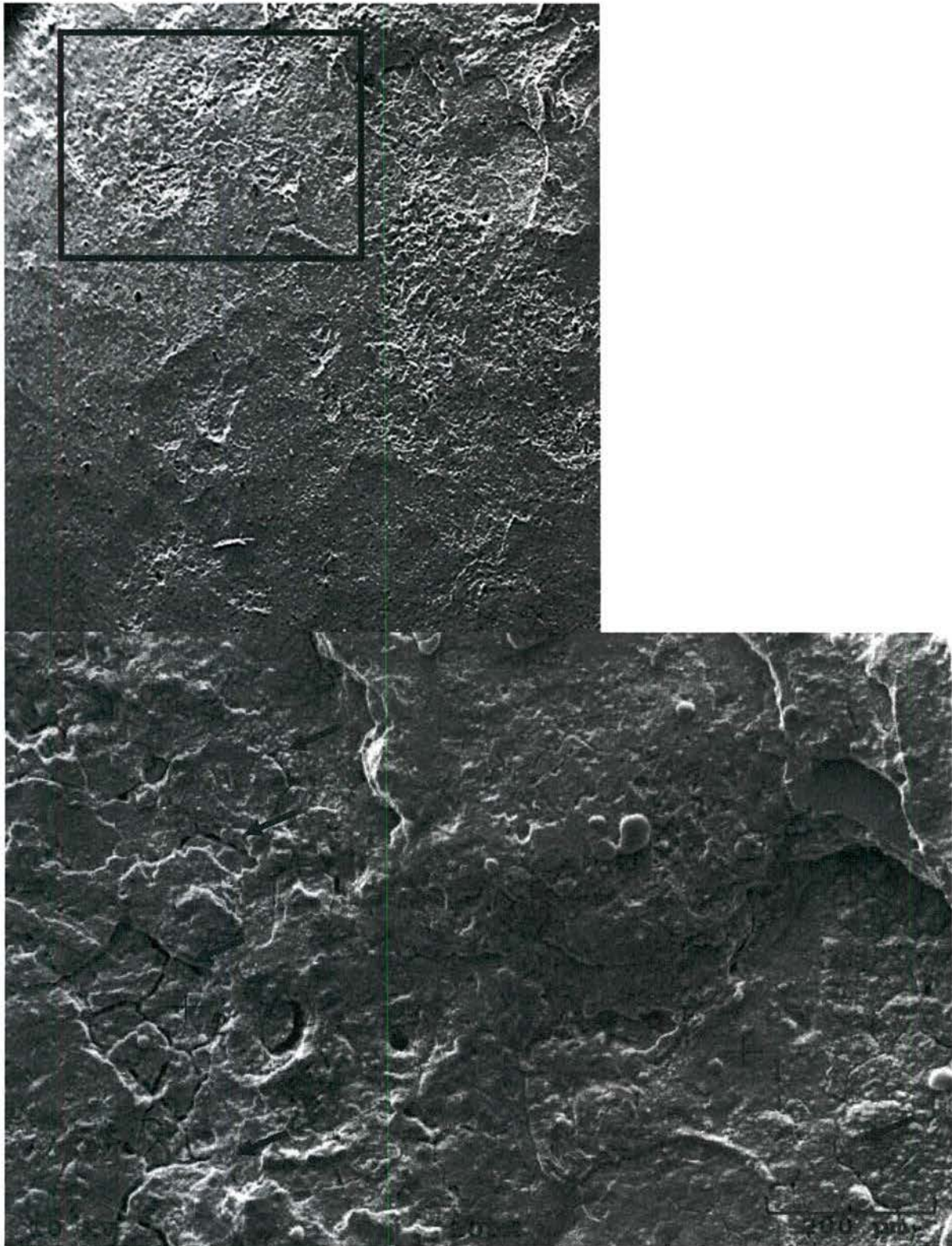
Figure 48 - Higher Magnification SEM photomicrograph of Surface Oxide from Torsion Bar 53-2 (Mag 100x)
