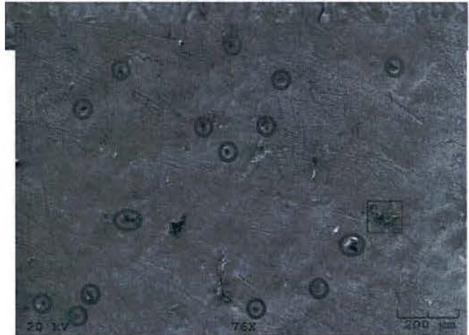
Figure 182 - SEM Photomicrograph of Laser Cleaned Surface (Mag 76x)
