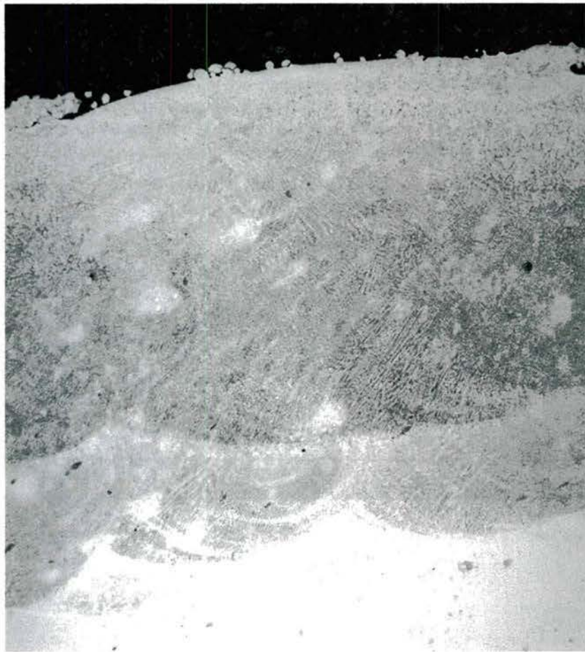
Figure 83: 50x image of optimal settings for 9310H Alloy Steel
