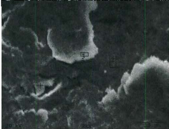
Figure 154 - SEM Photomicrograph of Torsion Bar 7 after Glass Bead Blasting (Mag 2000x)
