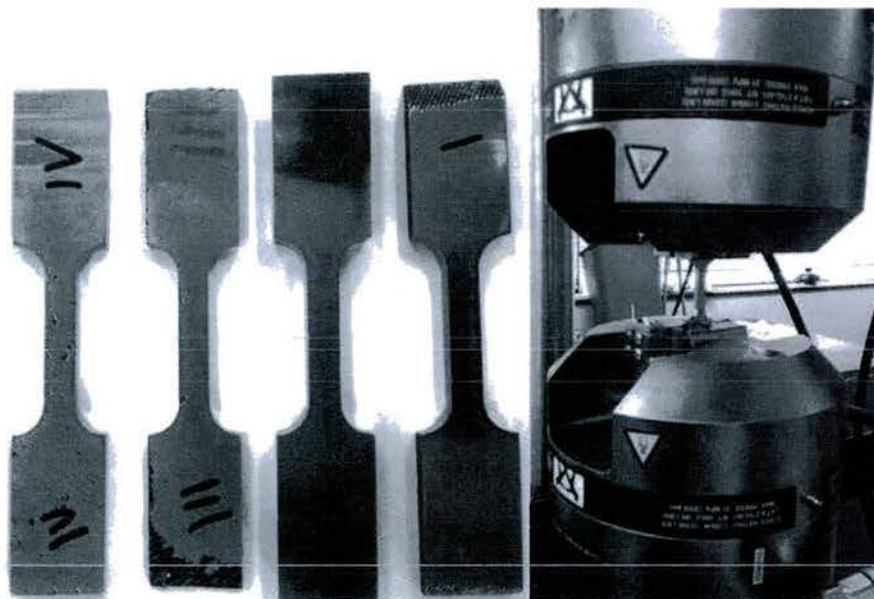
Figure 88: Tensile testing of coatings
