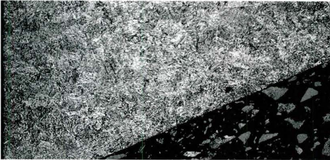
Figure 180 - Cross-Sectional Optical Photomicrograph of Torsion Bar L-3 – Coating Removal Only- 2% Nital Etch (Mag 200x)
