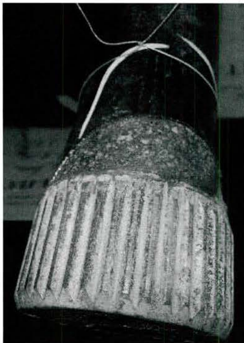
Figure 98 - Coating Disbond and Corrosion on Rejected AAV Torsion Bar
