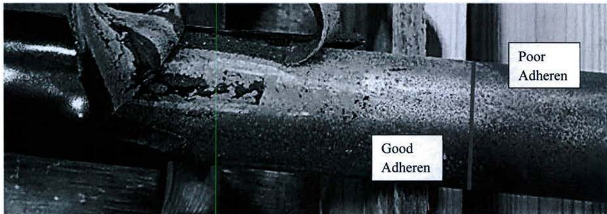
Figure 65 - Transition from Poor to Good Coating Adherence
