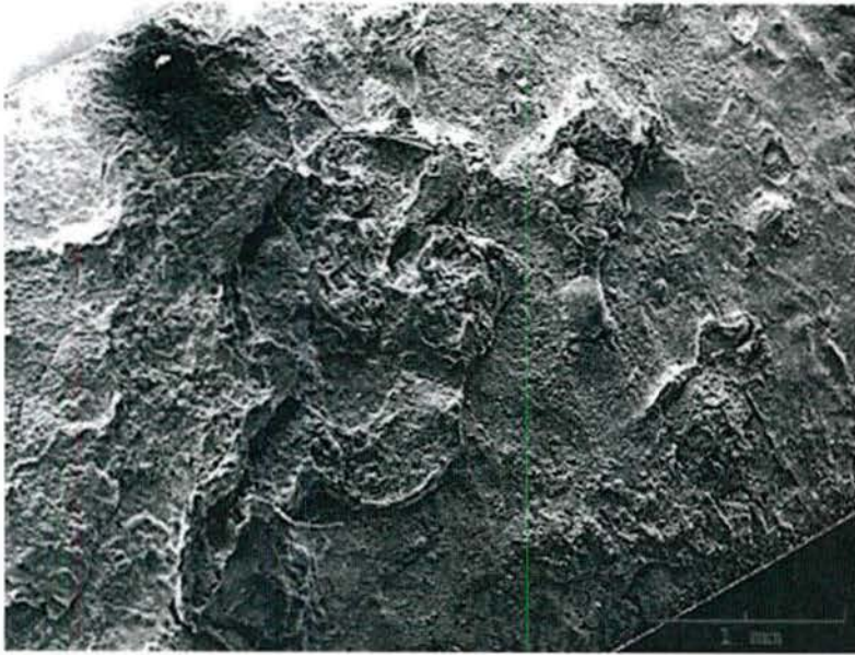
Figure 43 - SEM Photomicrograph of the Corrosion on Torsion Bar 55-2
