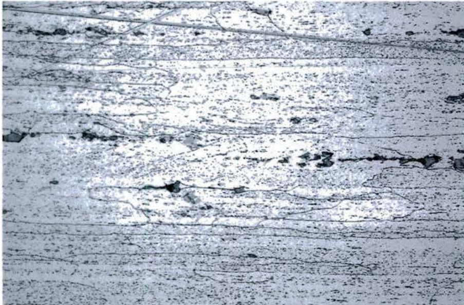
Figure 17 - Optical Photomicrograph -5083 Microstructure, Region 1 after 40% Phosphoric Acid Etch (Mag 500x)
