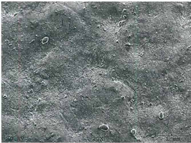
Figure 32 - SEM Photomicrograph of Surface after Wire Brush Cleaning (Mag 20x)
