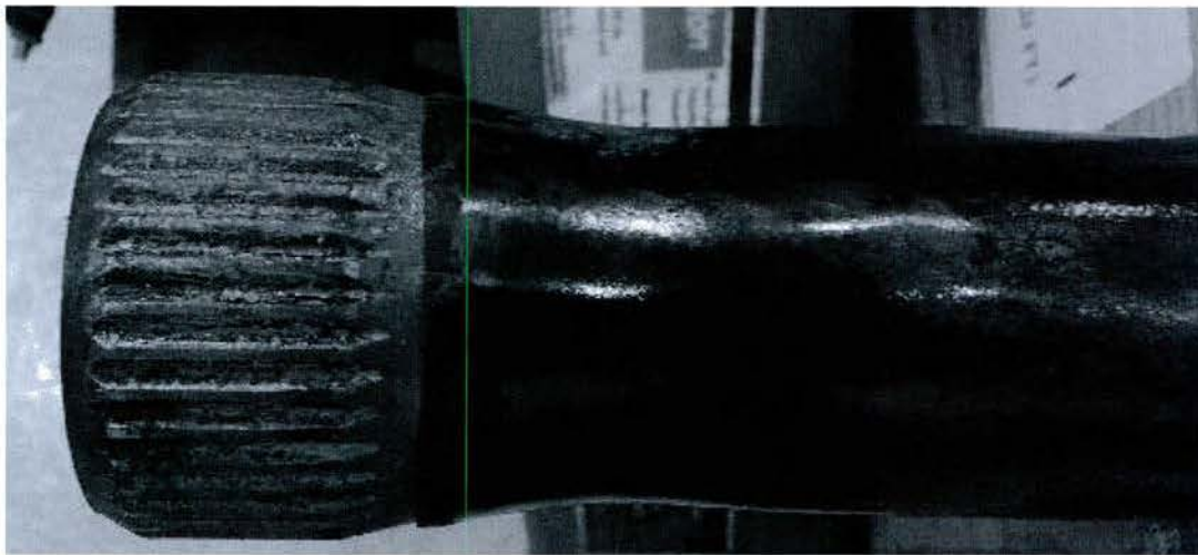
Figure 62 - Torsion Bar Send from Albany Depot Exhibiting Coating Disbonding
