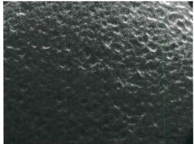
Figure 152 - SEM Photomicrograph of Torsion Bar 7 after Glass Bead Blasting (Mag 20x)
