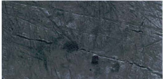
Figure 183 - SEM Photomicrograph of Laser Cleaned Surface (Mag 234x)
