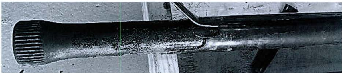
Figure 83 - Coating Easily Removed Revealing an Oily Film
