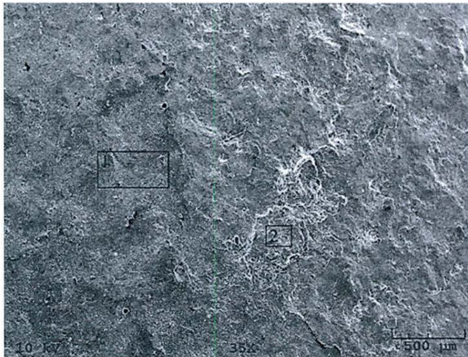
Figure 69 - SEM Photomicrograph of Surface Beneath the Coating in a Poor Adherent Region from Figure 65 (Mag 33x)
