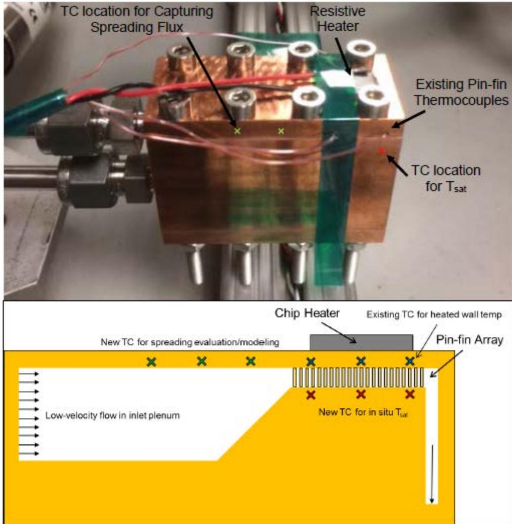
**Figure 23: Thermocouple Locations on the Micro Pin-Fin Cooler Manifold**
