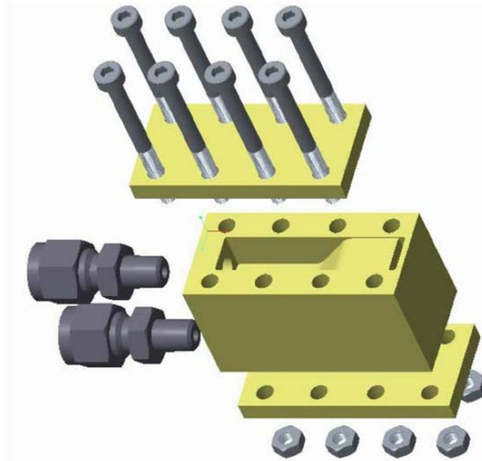
**Figure 11: Exploded View of Cryogenic Micro Pin-Fin Cooler**
