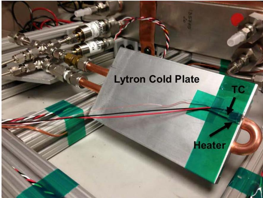
**Figure 16: Lytron Cold Plate Setup used to Test LN<sub>2</sub> Flow Loop Apparatus**
