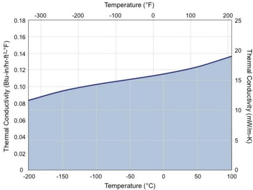
**Figure 14: Thermal Conductivity vs. Temperature for Cryogel Z Insulation**
