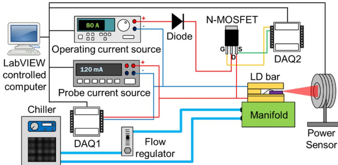
**Figure 38: Schematic Illustration of Junction Temperature Measurement Setup**
