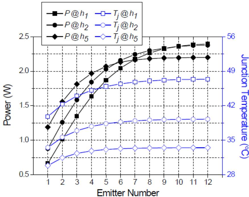
**Figure 63: Junction Temperature and Power of each Emitter in the Left Half of the LD Array at  $h_1, h_2,$  and  $h_5$**
