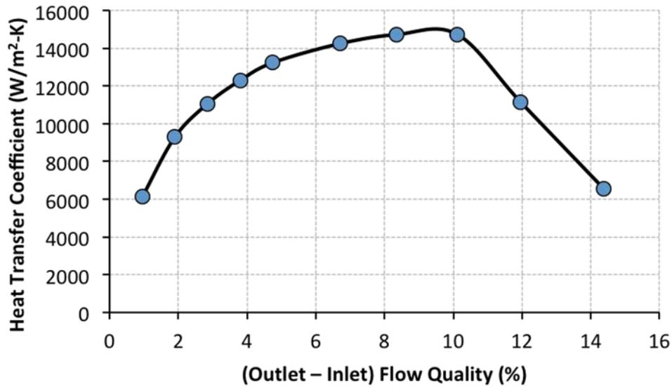
**Figure 17: Heat Transfer Coefficient versus Change in Flow Quality (outlet – inlet) for Lytron Cold Plate with LN<sub>2</sub>**
