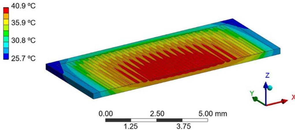
**Figure 53: Temperature Distribution of the LD Array**
