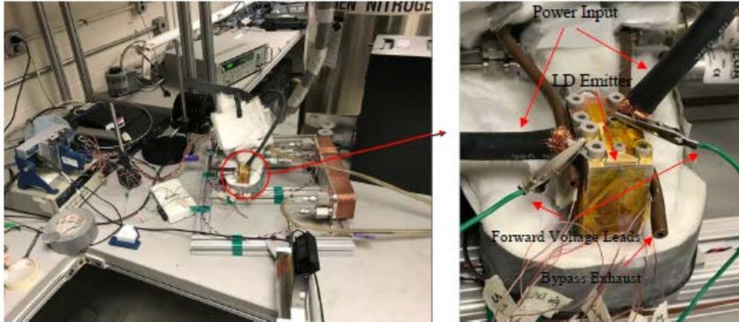
**Figure 30: Nitrogen Flow Loop with DILAS LD Bar Mounted on Micro-Pin Fin Cooler**
