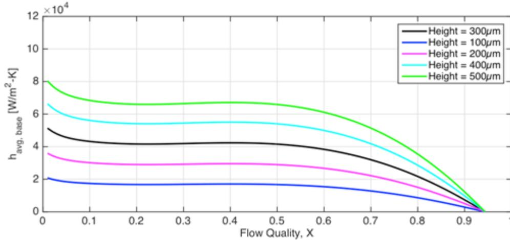
**Figure 2: Influence of Pin Fin Height on the Base Heat Transfer Coefficient vs. Flow Quality Profile for a Mass Flux of  $800 \text{ kg/m}^2\text{-s}$  and Pin Height of 100, 200, 300, 400, and 500  $\mu\text{m}$**
