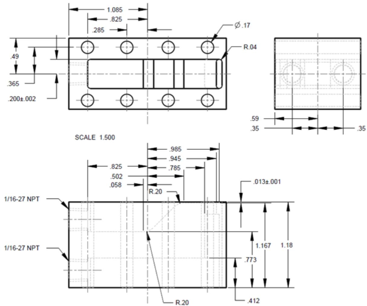
**Figure 22: Central Manifold Block Dimensions (inches)**
