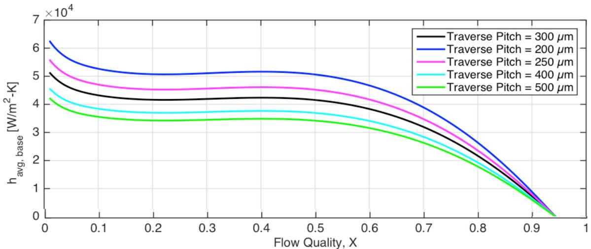
**Figure 4: Influence of Traverse Pin Fin Pitch on the Base Heat Transfer Coefficient vs. Flow Quality Profile for a Mass Flux of 800 kg/m<sup>2</sup>-s**
