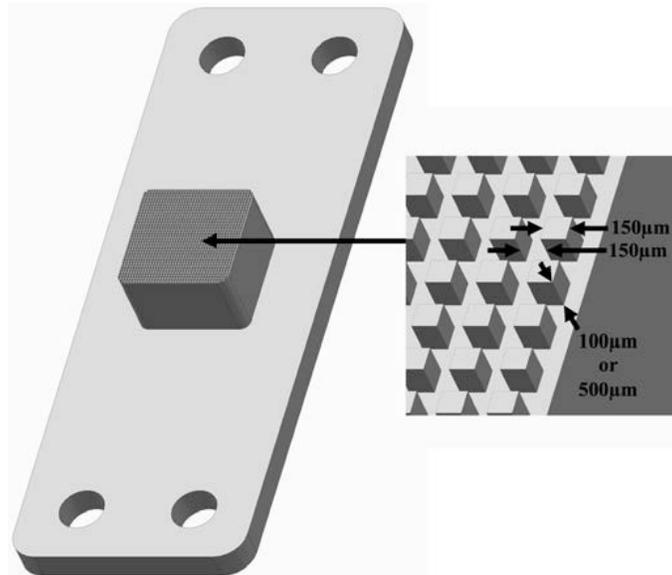
**Figure 6: Copper Micro Pin-Fin Channel**
