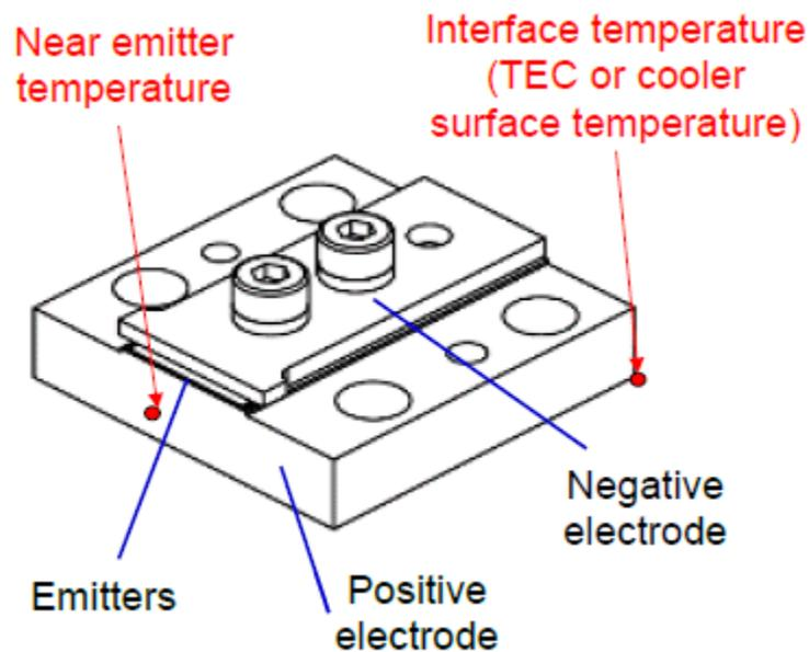
**Figure 29: DILAS Conduction Cooled Laser Diode Bar**
