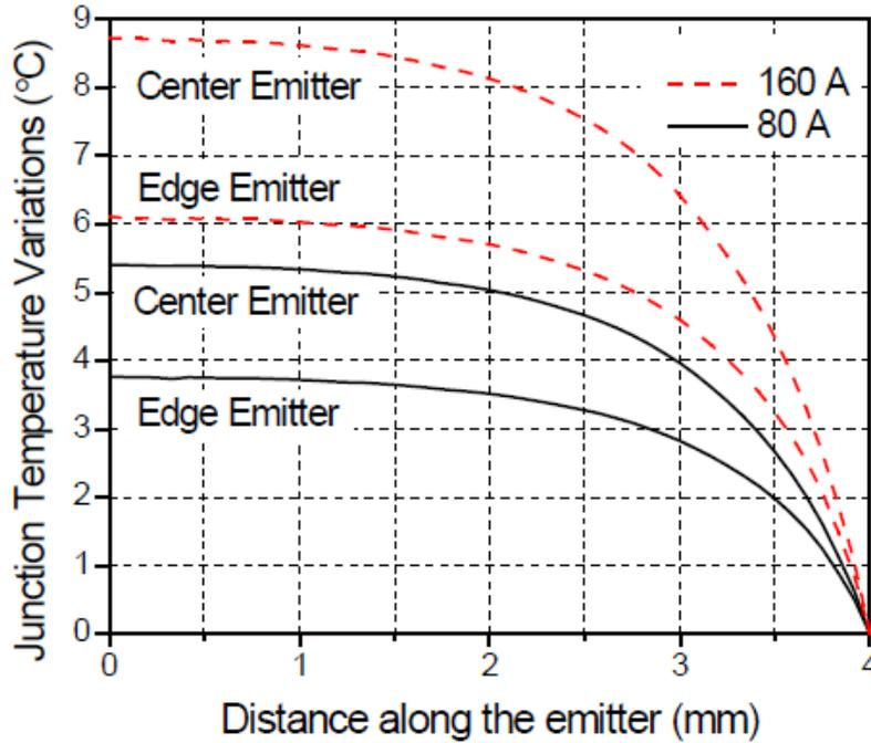
**Figure 47: Junction Temperature Variations along the Emitter**
