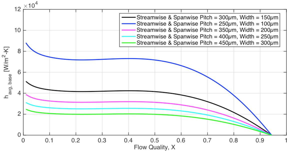
**Figure 5: Influence of Pin-Fin Width on the Base Heat Transfer Coefficient vs. Flow Quality Profile for a Mass Flux of  $800\ \text{kg/m}^2\text{-s}$  and Constant Gap of  $150\ \mu\text{m}$  between Adjacent Pins**
