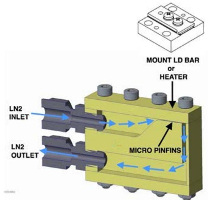
**Figure 10: Cross-Sectional View of Cryogenic Micro Pin-Fin Cooler**
