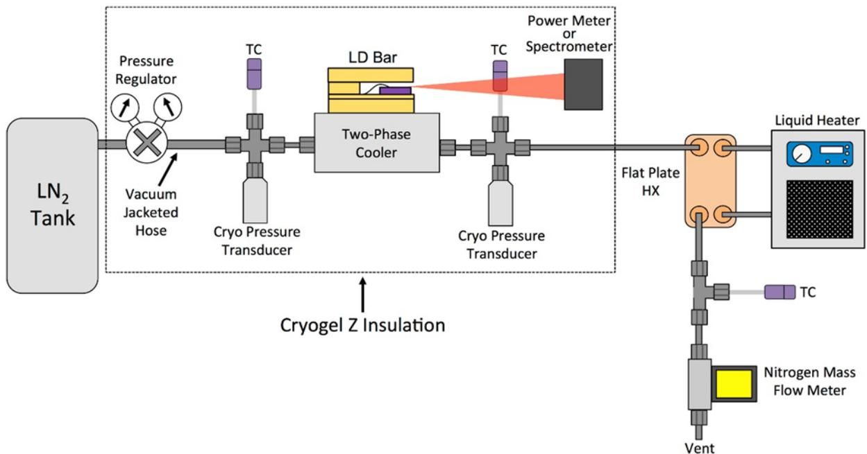
Figure 13: Schematic of LN<sub>2</sub> Flow Loop Apparatus
