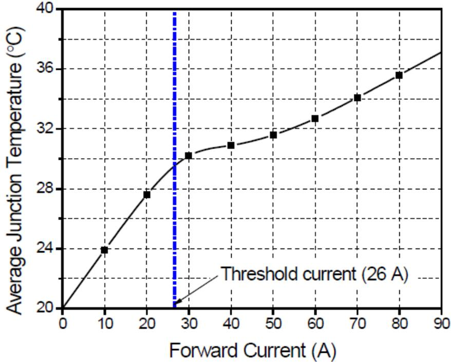
**Figure 42: Average Junction Temperature at different Forward Currents**
