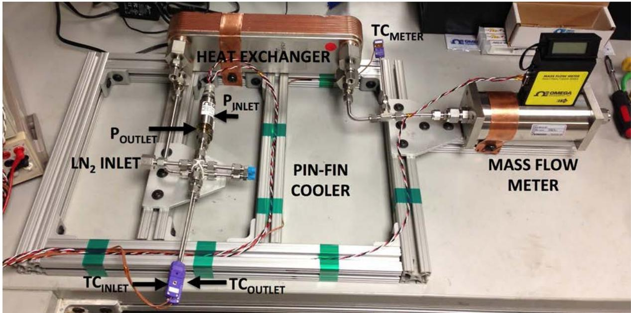
Figure 12: Assembled LN<sub>2</sub> Flow Loop Apparatus
