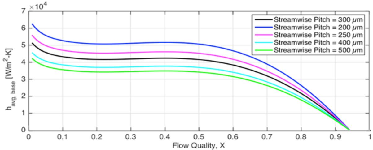
**Figure 3: Influence of Streamwise Pin Fin Pitch on the Base Heat Transfer Coefficient vs. Flow Quality Profile for a Mass Flux of 800 kg/m<sup>2</sup>-s**
