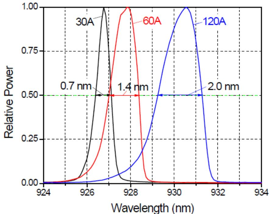
**Figure 48: Normalized Power Spectrum at 30, 60, and 160 A**
