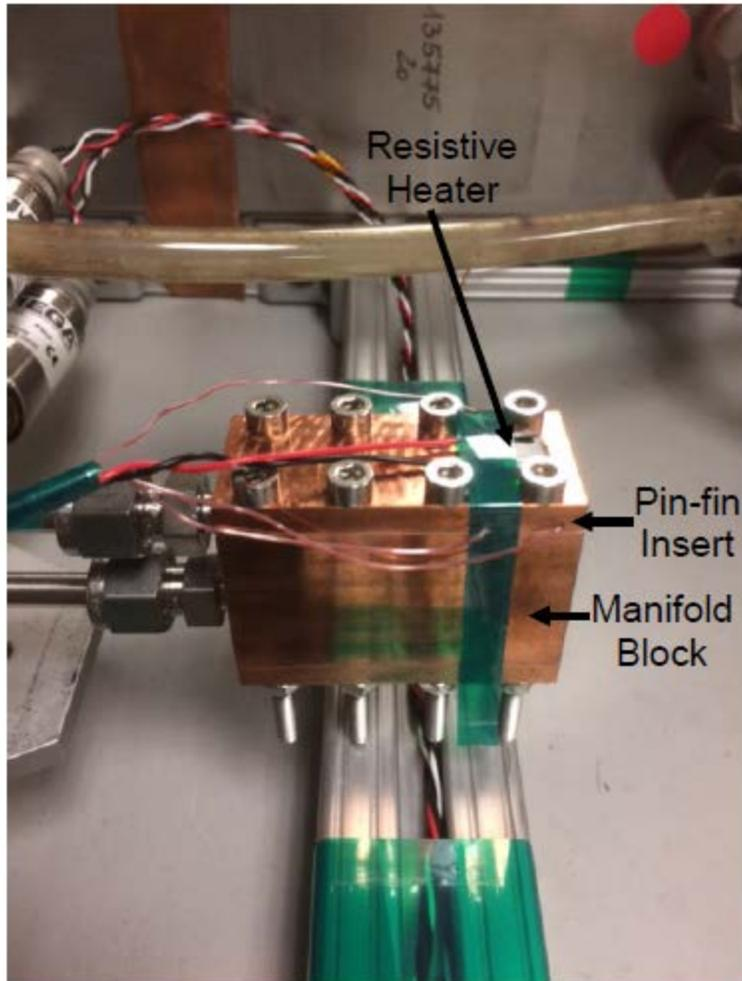
**Figure 18: Assembled LN<sub>2</sub> Pin-Fin Cooler**
