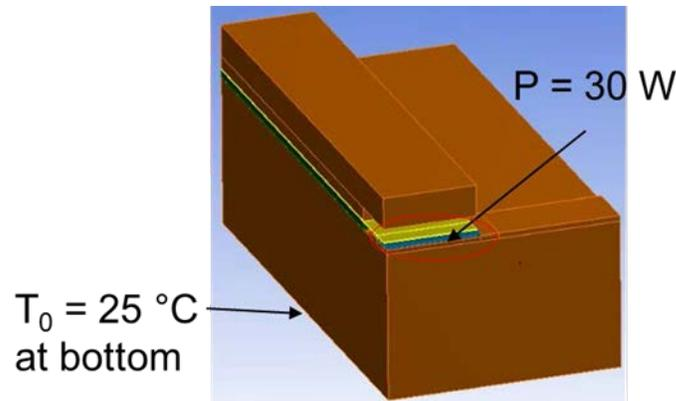
**Figure 68: Loading and Boundary Conditions for the Thermal Model**
