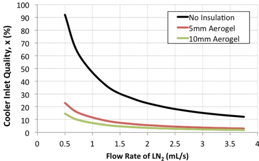
**Figure 15: LD Cooler Inlet Quality versus Flow Rate from Heat Leakage Approximation for LN<sub>2</sub> Flow Loop Apparatus**
