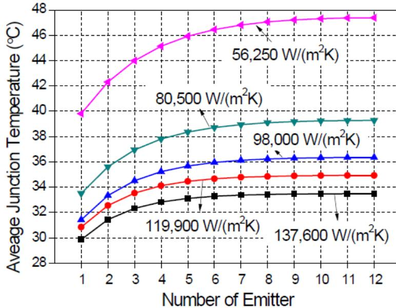
**Figure 54: Average Junction Temperature of each Emitter in the Left Half (symmetry) under various Heat Transfer Coefficients**
