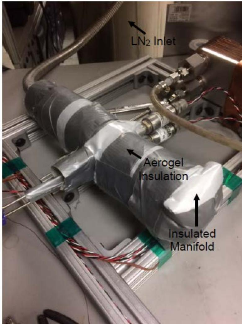
**Figure 19: Flow Loop and Manifold Aerogel Insulation**
