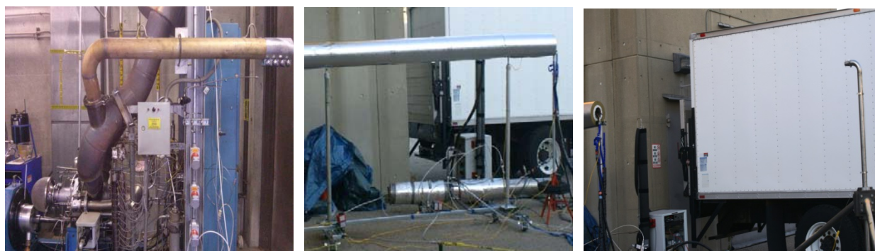
Figure 5. T63 Engine with Extension Pipe to Direct Exhaust Outside of the Test Cell for Exhaust Sampling with Tip-diluted and Gas Probes at Pipe Exit and Large Gas Probe at Plume
