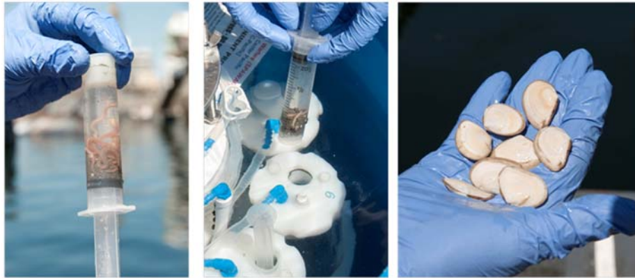
Figure 2.2. Smaller Organisms (e.g. Polychaetes and Amphipods) Are Delivered by Preloaded Syringes while Larger Organisms (e.g. Clams) Are Placed into Chambers Prior to Deployment.
