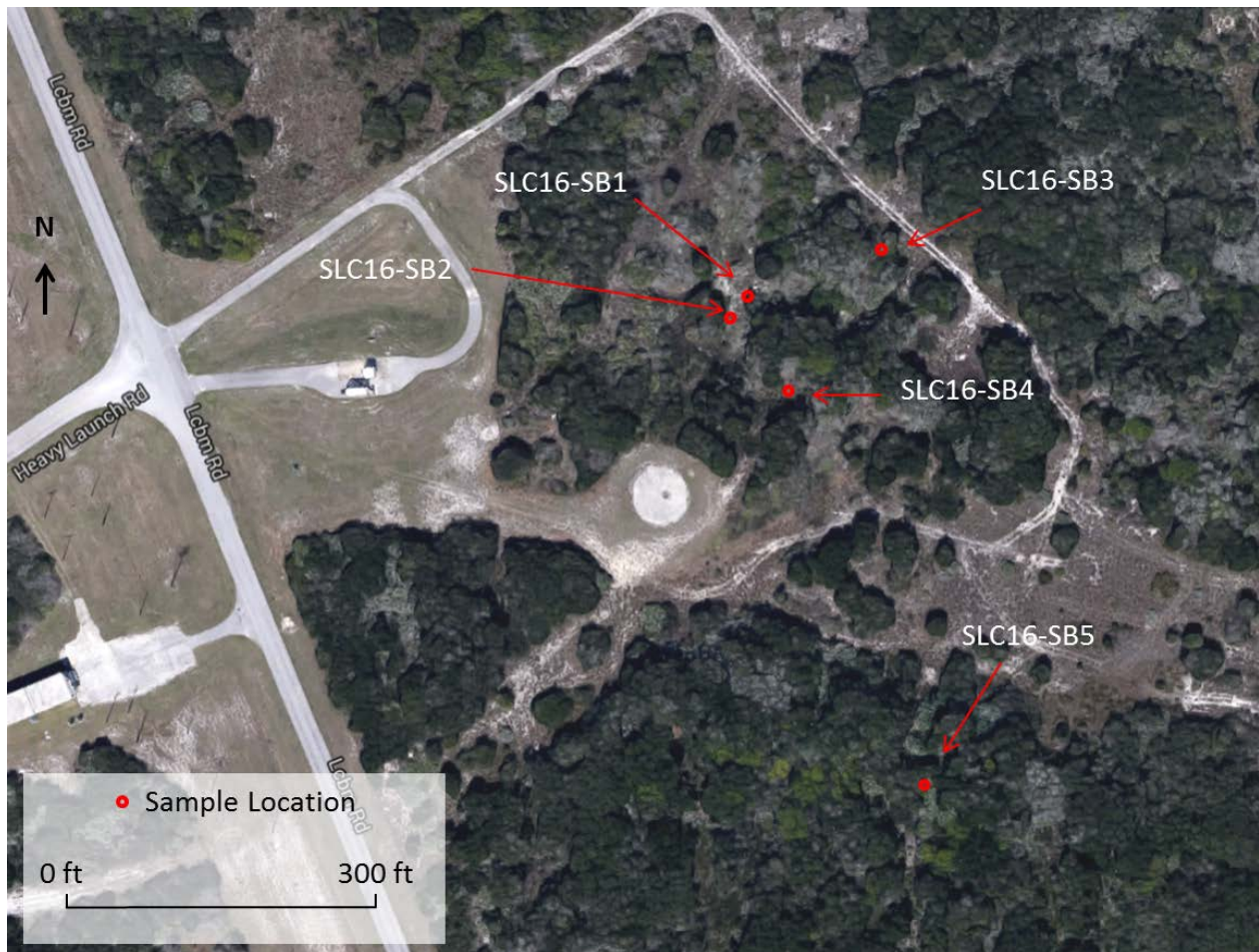
Figure 102. Locations for Investigation Points at SLC-16, Cape Canaveral Air Force Station. At each location, vertical profiling, soil sub-sampling, and groundwater sampling was completed. Source area is in vicinity of locations SLC16-SB1 and SLC16-SB2. Groundwater generally flows in southeast direction.
