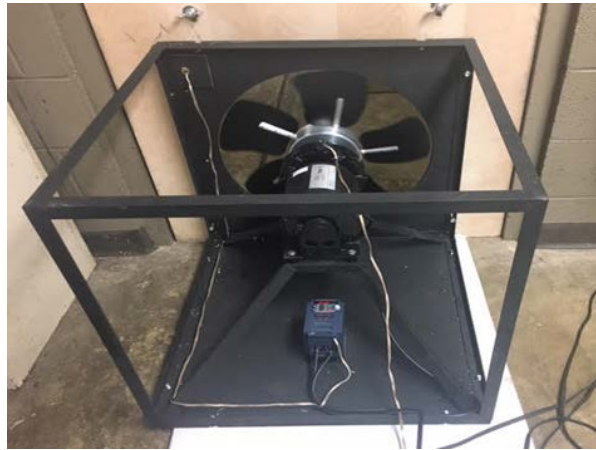
Fig. 7 Rotary subwoofer speaker mounted to wooden door
