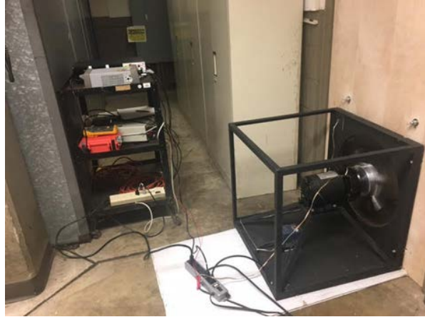
Fig. 6 Setup of rotary subwoofer attached to a wooden door, with the waveform generator and amplifier in plain view (top shelf of cart)
