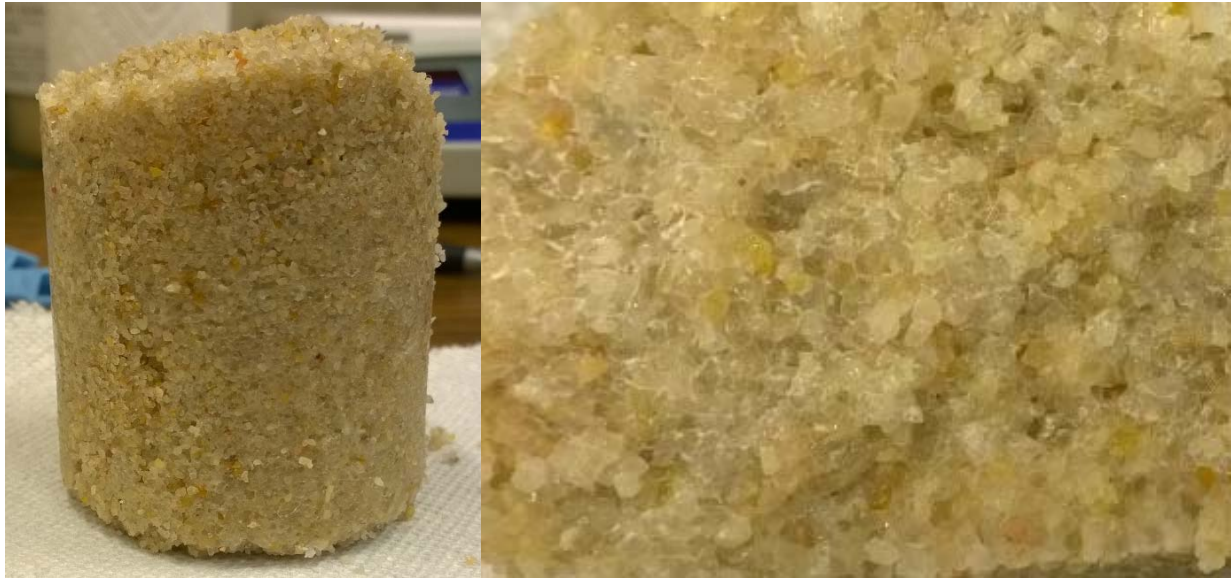
Figure 3. Extracted #2 filter sand from falling head columns.
