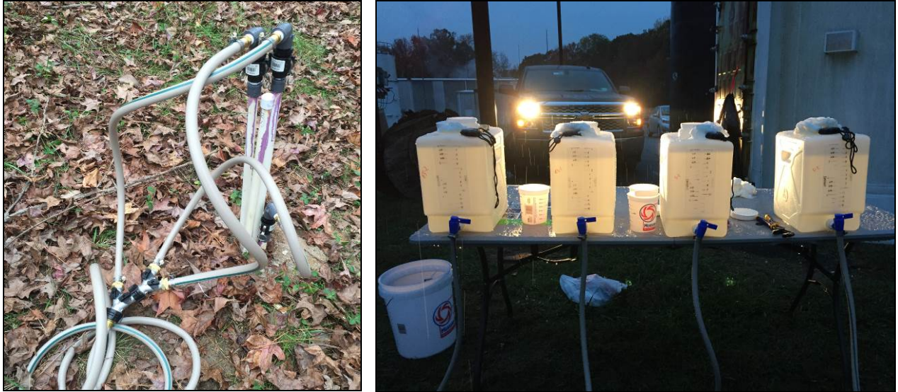
Figure 6.4: Well Head Injection Assemblies (Left) and Water Vessels Setup for the Constant-Injection Test
