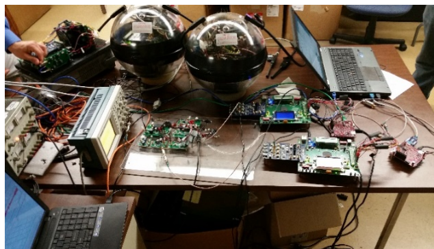
Figure 3. Photo showing two SSC Pacific software-defined modems tested in the laboratory with JANUS code.
