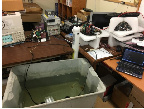
Figure 11. Photo showing test tank with SSC Pacific modem transducers.
