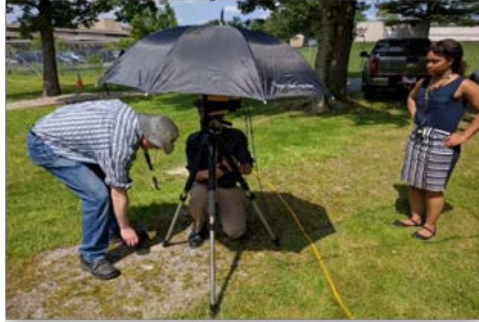
Fig. 8 Umbrella compensates for LDV overheating during test run
