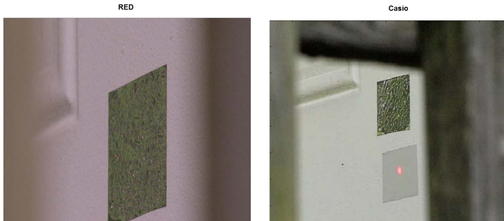
Fig. 9 Door experiment: speaker at 19 Hz, visual image through camera lens: RED (left), Casio (right)
