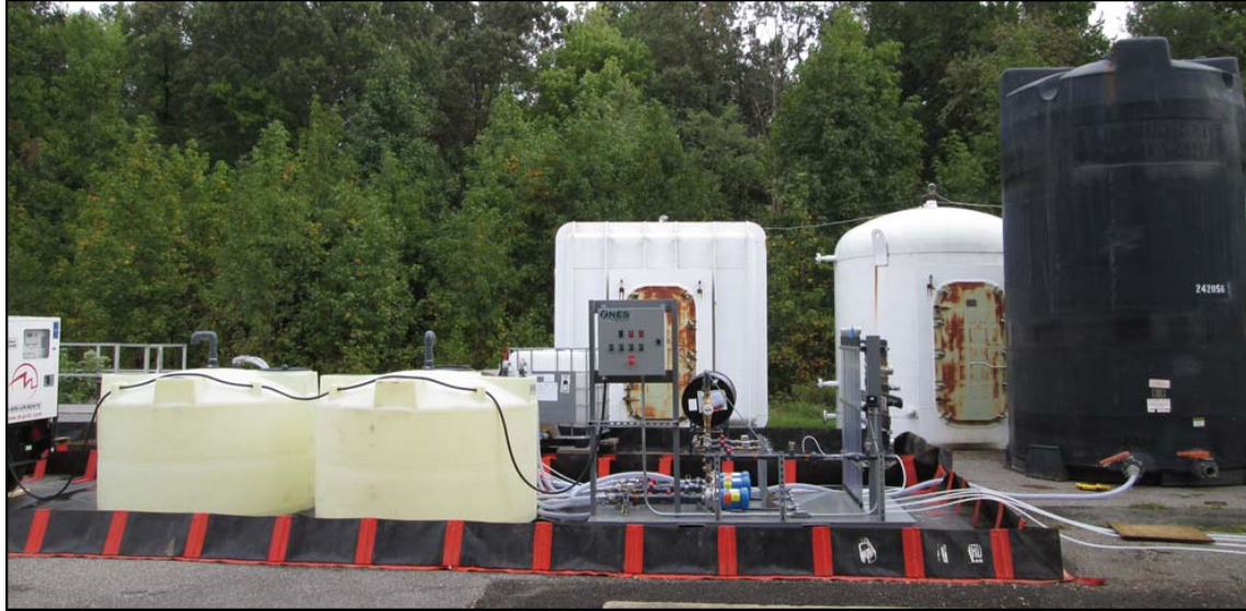
Figure 6.3: Injection Skid Assembly with all Components
