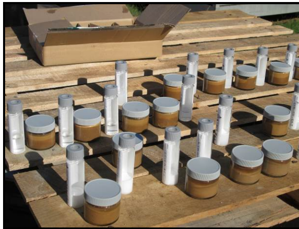
Figure 6.1: On-Site Gel Tests with Site Soils
