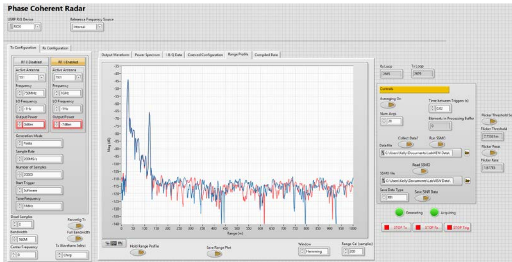
Fig. D-1 LabVIEW user interface for control of the software-defined radio (SDR) and processing received data. The left panel controls transceiver (Tx) and receiver (Rx) channel configuration. The middle panel selects the displayed data. The right panel controls various data monitoring operations.
