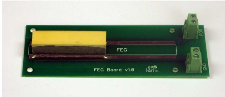
**Fig. 2 FEG surface mount soldered to circuit board**
