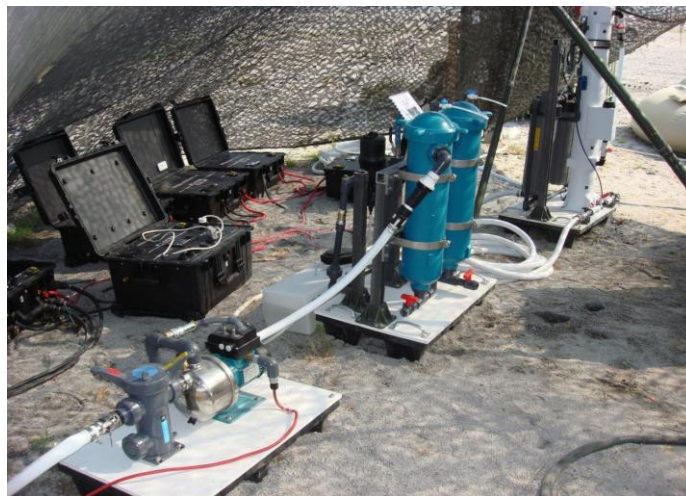
Figure 7: STAESS supporting the First Response Water Purifier at Crow Valley
