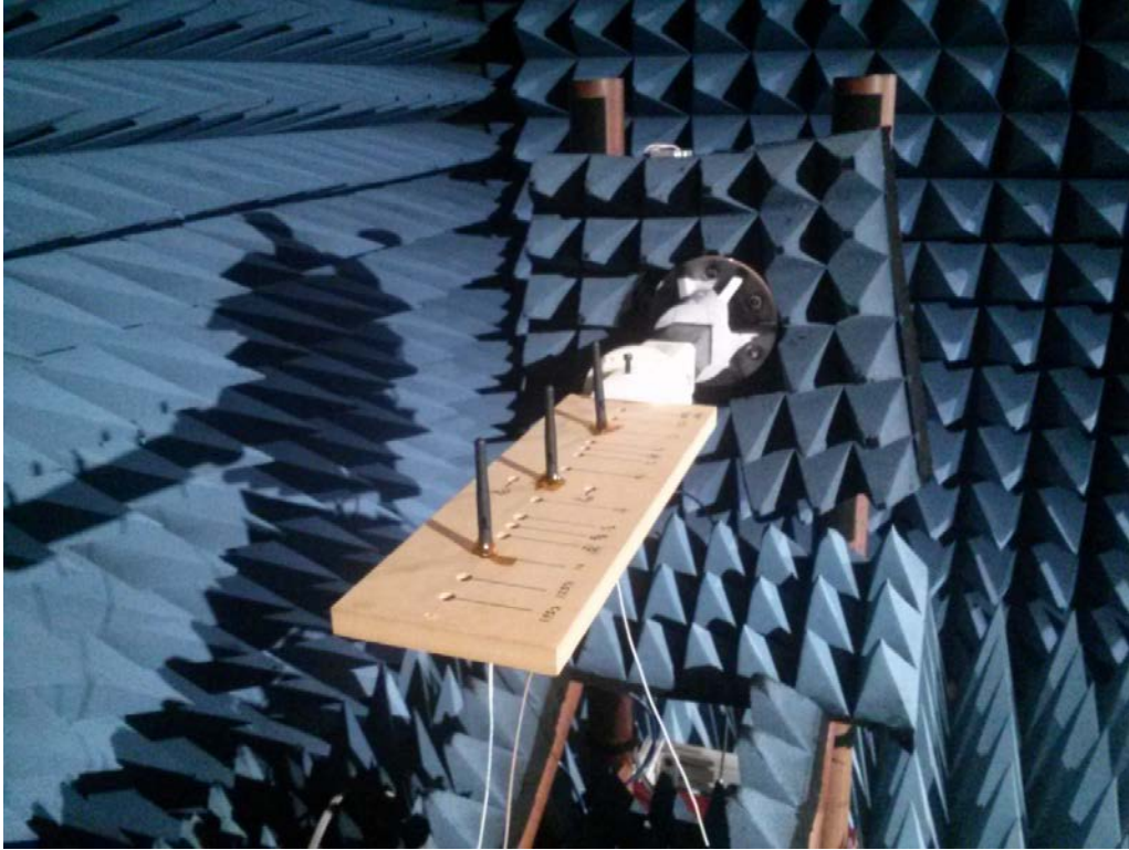
Fig. 15 Close-up of an example antenna array. The antenna in the middle is used for a calibration process described later.
