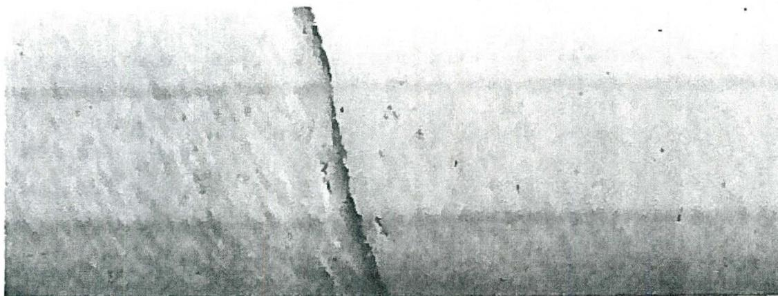
Fig. 25. Discontinuity in thermal structure of ocean surface and cold (black) whitecaps recorded by AN/AAD-2. Date: 21 Nov 1961; Time: 1935 R; Coordinates:  $39^{\circ}20'N$ ,  $71^{\circ}55'W$ ; Aircraft altitude: 2000 ft; Detector: InSb, square, 2.5 by 2.5 mm; Length of area shown: 4.5 n mi.
