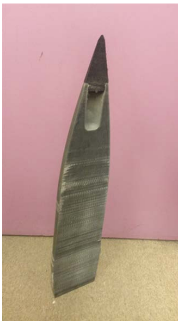
Figure D-supplemental 1. One-half of munition surrogate produced from intact 155-mm replica.
