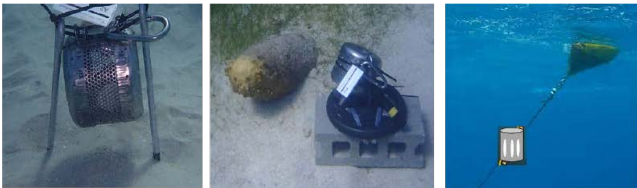
Figure 4. Deployment options for POCIS at a UWMM site including (left) screw anchors holding a POCIS sampler in place above sea floor using a grid (non-biased) deployment option; (center) placement of POCIS on a weighted brick system near potential leaking UWMM; or (right) using a mooring system in water column, potentially eliminating the requirement for cost and safety factors associated with munitions response divers.
