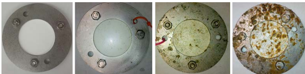
Figure 2-7. Representative pictures of POCIS membranes upon initiation of 7-day MC spike laboratory experiment following deployment at Gulf Breeze East Dock (from left to right), for 0, 7, 14, and 28 days during July 7 to August 4, 2015.
