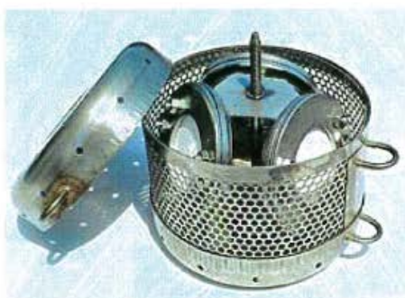
Figure 3. Commercially available stainless steel canister that will be used to house the POCIS passive samplers. The Composition B fragment will also be contained in one of these canisters and secured to pier with DoD identification tags. http://www.est-lab.com/pocis.php
