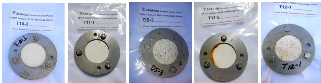
Figure 5-14. Representative appearance of sampler membranes after 19–23 days of deployment.
