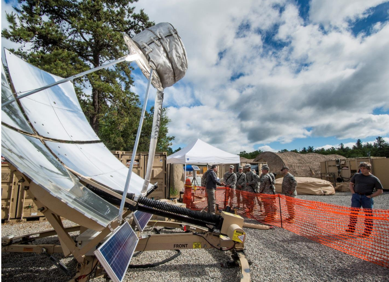
Figure 4: Self-Powered Solar Water Heater (SPSWH)
