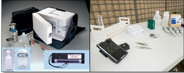
Figure 32: WQM-PM. Left: the current field 24-h incubation; right: cell phone-based pathogen detection kit
