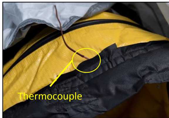
Figure 91: Thermocouple in MILHUT Air Duct
