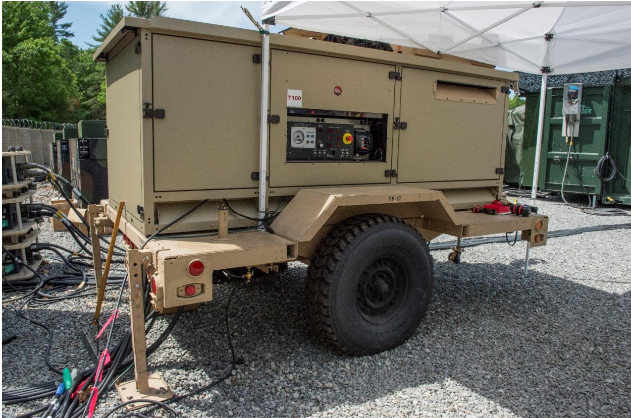
Figure 6: HMMWV-Towable Load Following 100Kw Power Unit (T100)
