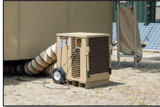
Figure 10: Air Conditioner for SLiM
