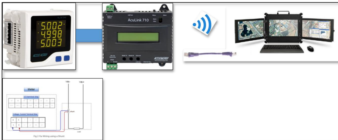
Figure 62: Accuenergy DC Meter High Level Setup
