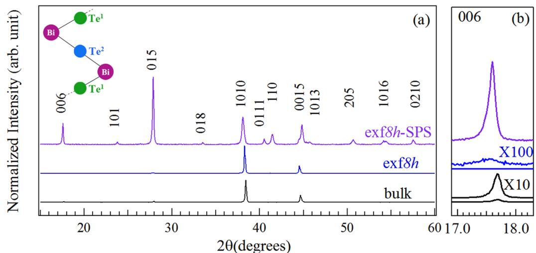
**Figure 1.** X-ray diffraction patterns. **(a)** Bulk  $n$ -type  $\text{Bi}_2\text{Te}_{2.7}\text{Se}_{0.3}$  sample compared to the 8-hr exfoliated flake before and after SPS with a  $\text{Bi}_2\text{Te}_3$  quintuple as inset; **(b)** (006) peak suppressed in the exf8h (X100), but more pronounced in the exf8h-SPS.
