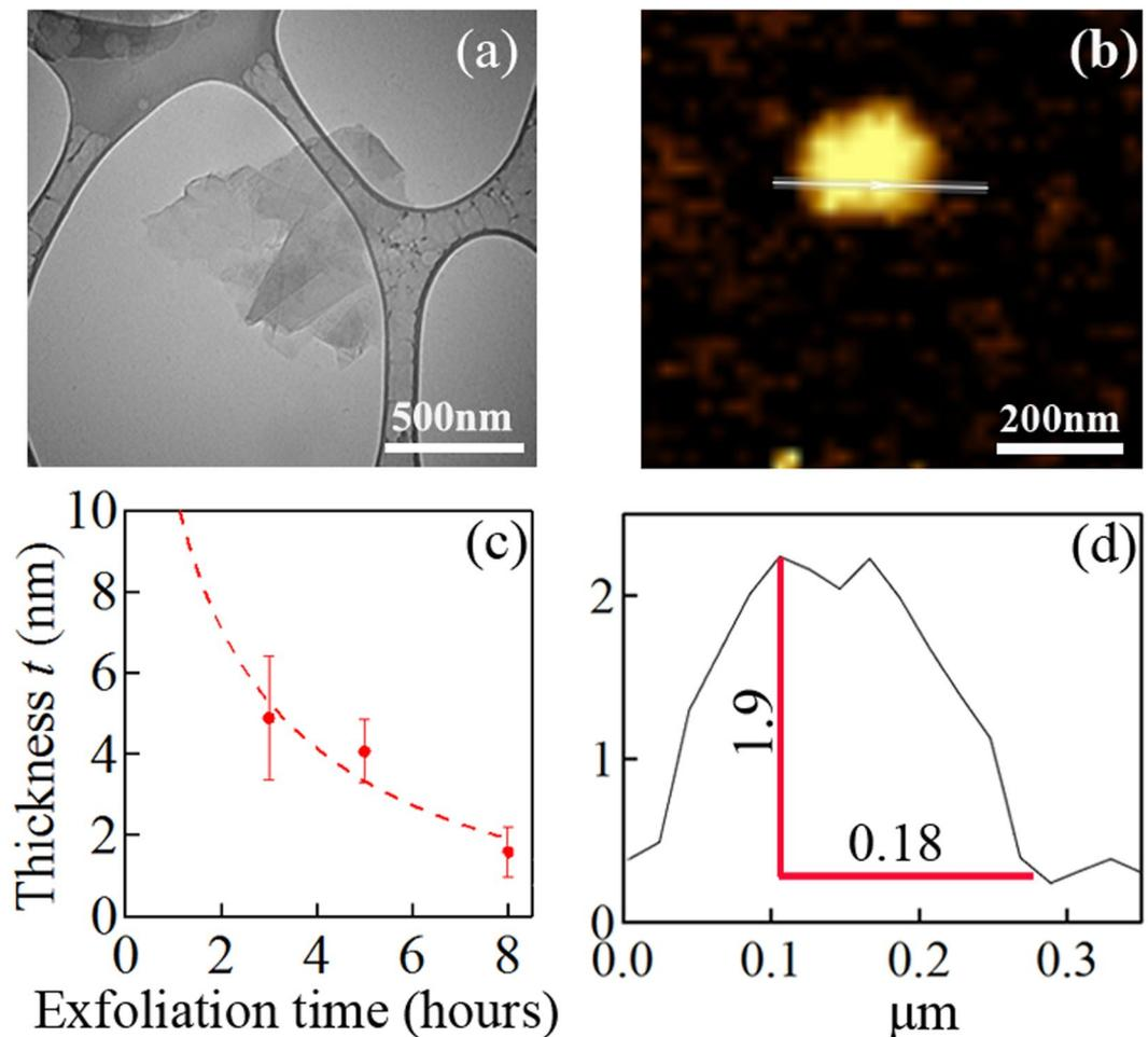
**Figure 2.** Representative TEM (a) and AFM (b) images of the exf8h sample. (c) The average thickness of the exfoliated *n*-type Bi<sub>2</sub>Te<sub>2.7</sub>Se<sub>0.3</sub> flakes as a function of exfoliation times (0 h, 3 h, 5 h, and 8 h). The full width of half maximum of thickness distribution (Gaussian distribution) were used as error bars. *t* tends to be infinite at 0 h and the dash line is a guide to the eye. (d) The lateral size and height of a representative flake shown in (b).
