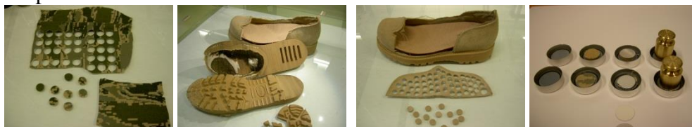
Figure 47 Examples of test samples prepared from US Army clothing and boots.
