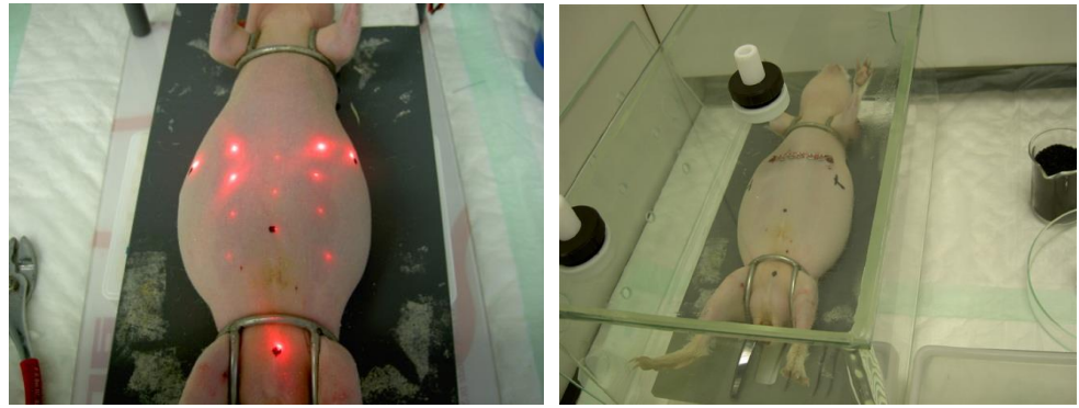
Figure 9 Experimental set up with laser beams that mark exposure sites on hairless guinea pig.
