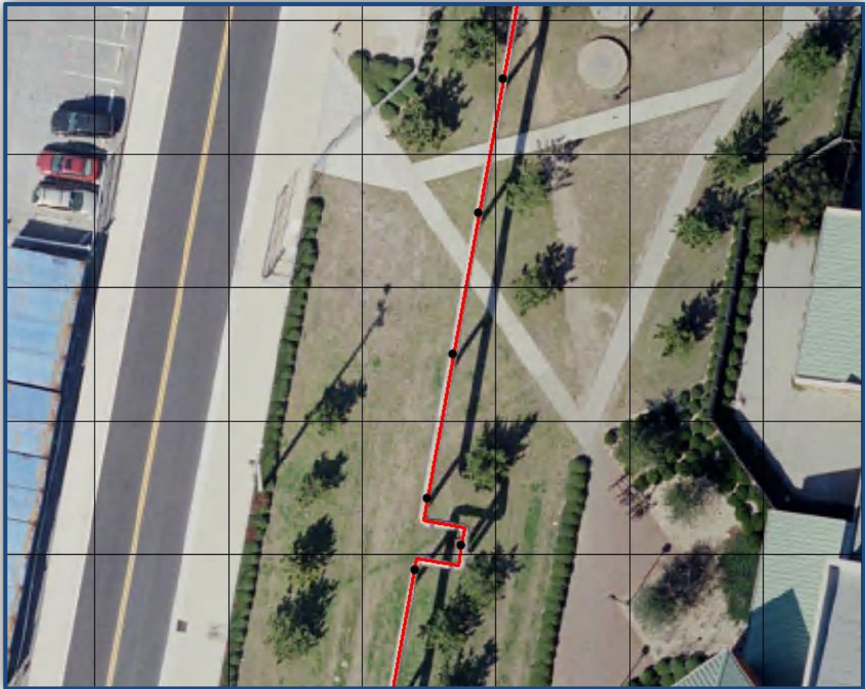
Figure 123. Example of the mapping products that have been generated by the study using the GIS-based ACN approach. Here, a small portion of the resource distribution system is represented in red, while supporting columns are represented as black dots.
