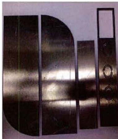
Figure 33. Aluminum plates fabricated by Waterjet Cutting
