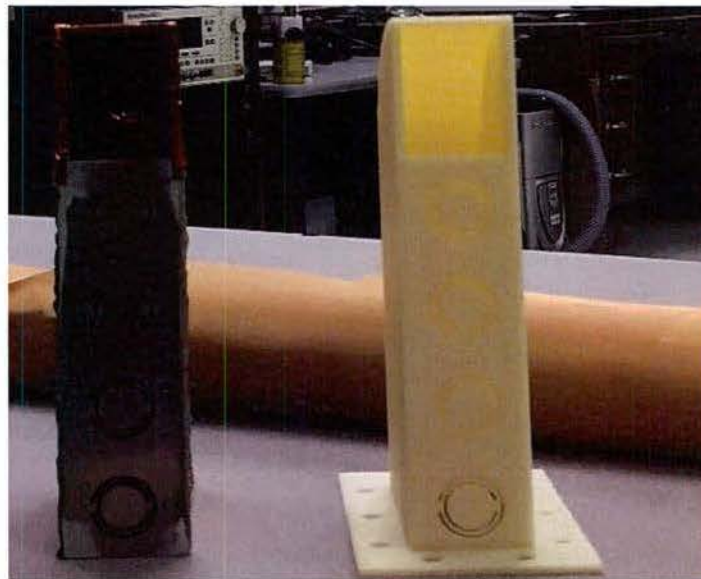
Figure 46. 3D printed CSR-SWA and aluminum CSR-SWA (on the right). Antenna one the left is the metallic version
