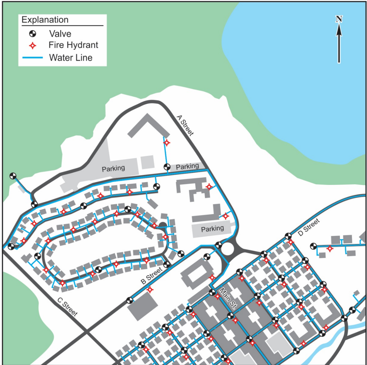
Figure 1.1. Typical Water Distribution System Layout for a DoD Installation
