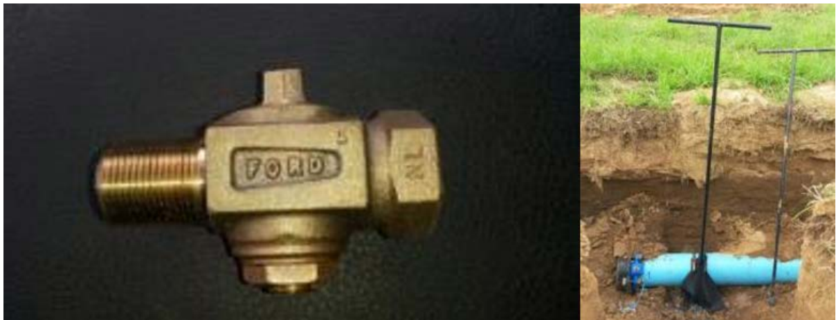
Figure 5.2. Simulated Leak Configuration Using Corporation Valves
