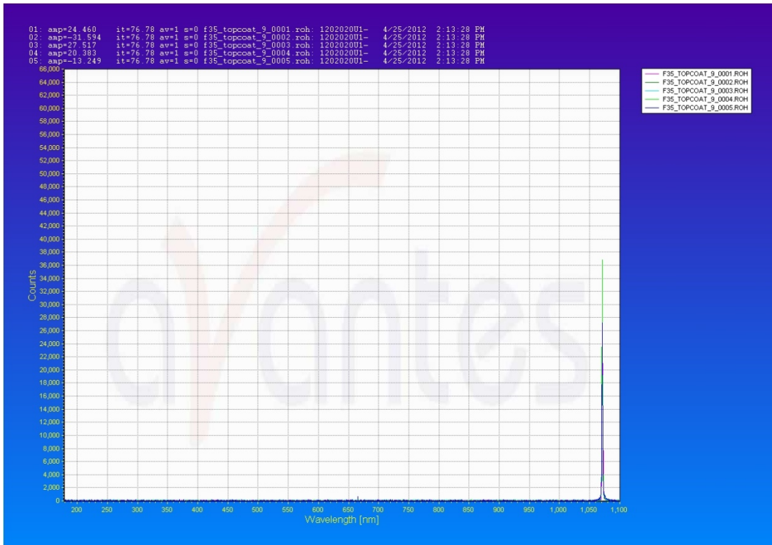
Figure 22. Topcoat Response at 540W (9% Laser Power)
