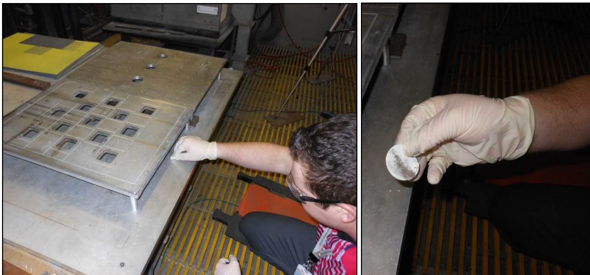
Figure 71. Baseline Wipe Sample Collected on Table Where Fiber Laser Stripping Process Occurs
