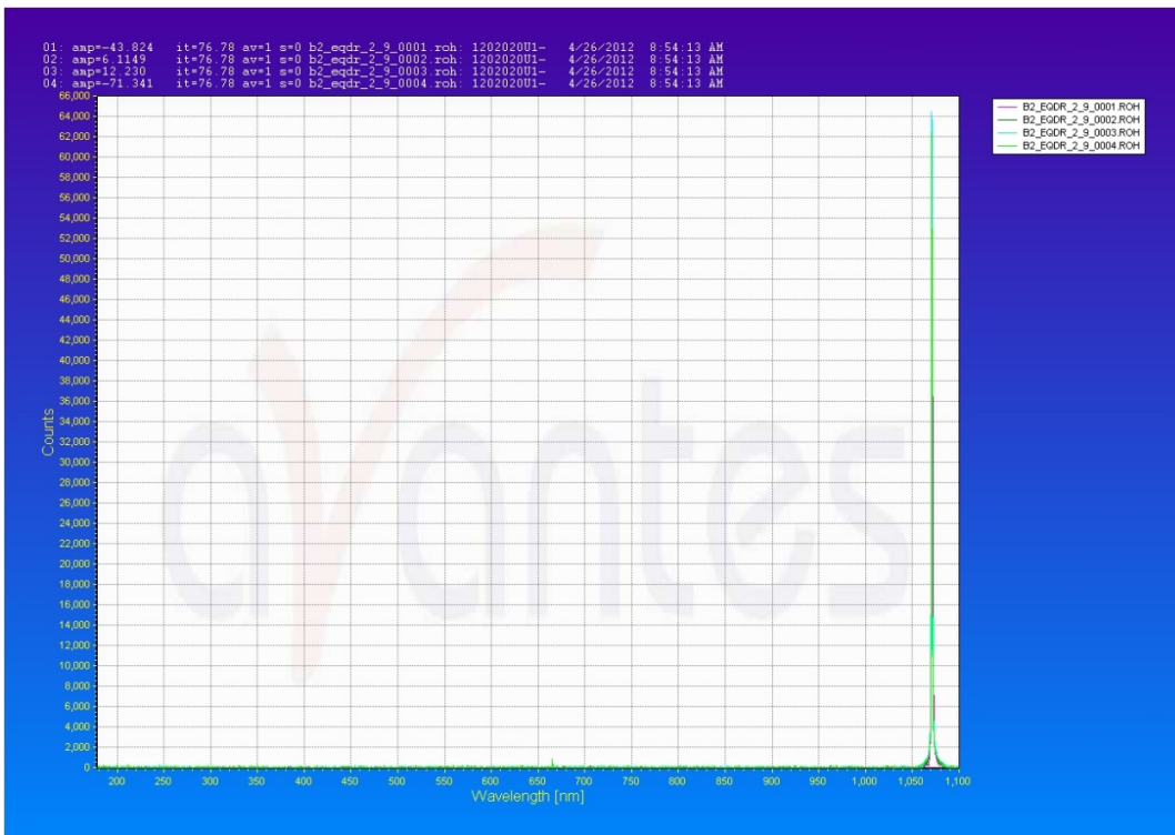
Figure 34. Response at 540W (9% Laser Power)
