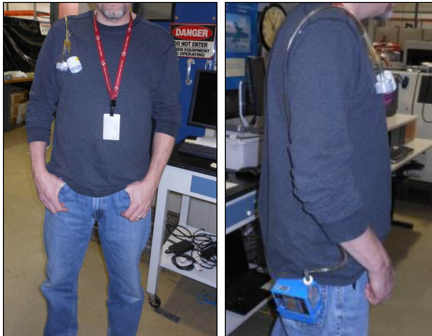
Figure 70. Personal Air Sample Located in the Operator's Breathing Zone
