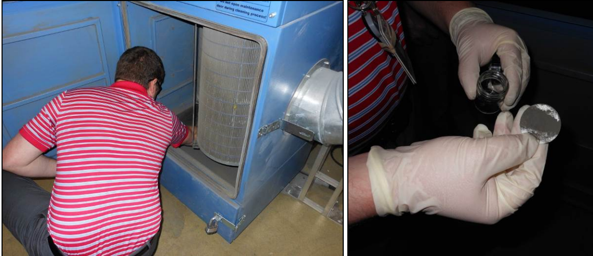
Figure 73. Wipe Sample Taken From TEKA Hopper after Laser Stripping
