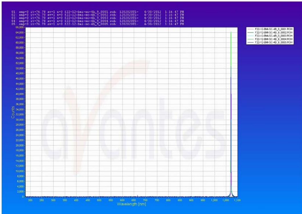
Figure 29. Intermediate Primer Response at 540W (9% Laser Power)
