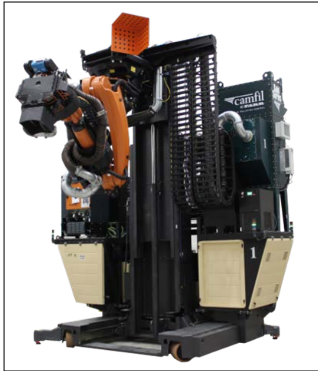
Figure 8. Advanced Robotic Laser Coating Removal System (ARLCRS)
