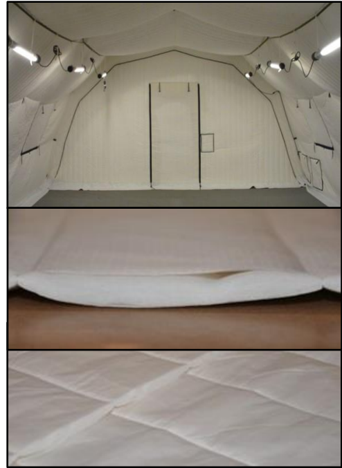
Figure C-49. Top to bottom: Non-Woven Composite Liner installed in an AS TEMPER shelter, non-woven composite fibrous batting, and manufacturing quilt lines
