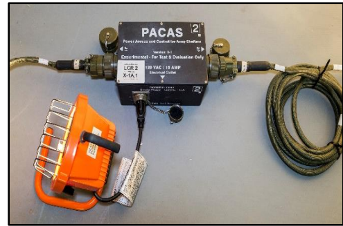
Figure C-9. Advanced Nanogrid Power Management (shown with a light set)
