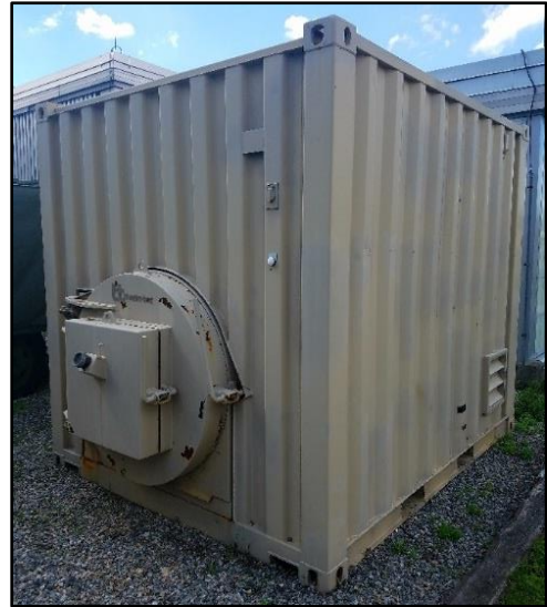
Figure C-72. Solid Waste Incinerator
