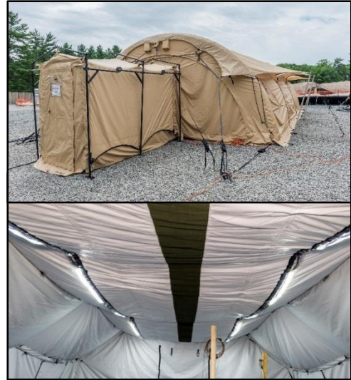
Figure C-19. Prototype Shelter System with V1.5 Liner
