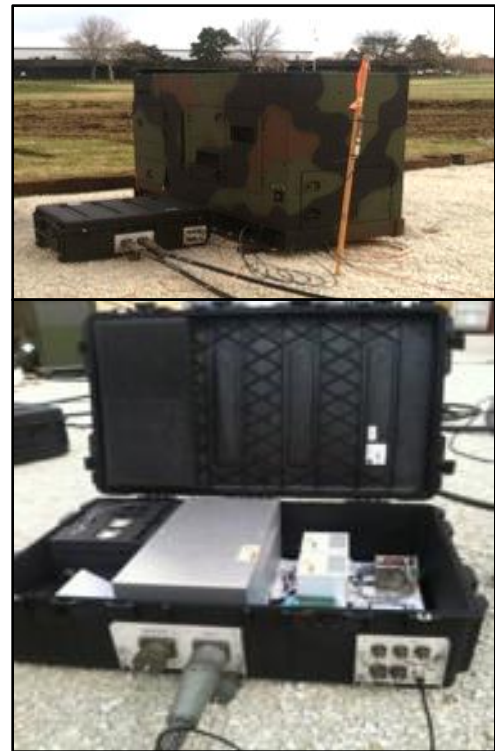
Figure C-16. DMMS interfacing with a generator set (top) and DMMS wireless metering solution (bottom)
