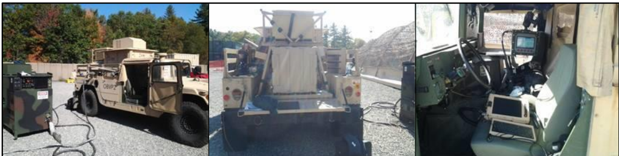
Figure 6: Bidirectional Onboard Vehicle Power/Tactical Vehicle-to-Grid Module
