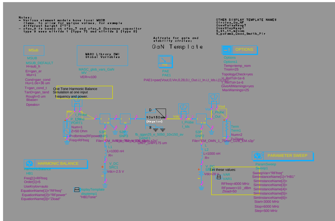
Fig. 33 ADS schematic of broadband amplifier with Momentum EM matching circuit simulations
