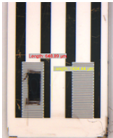
Figure 22: Sample film on a NanoSPR interdigitated electrode.
