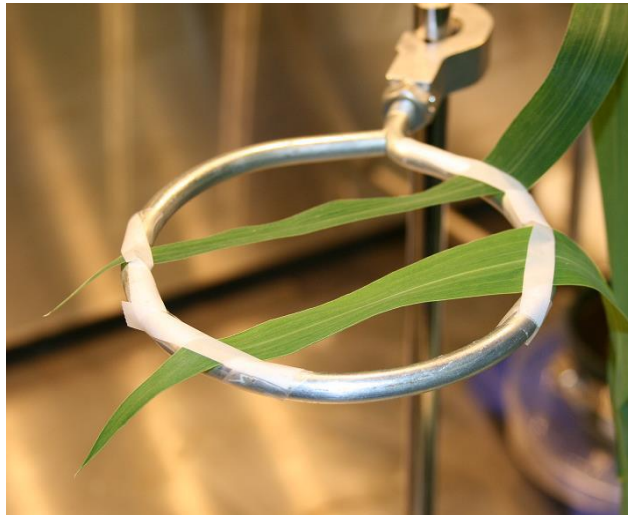
Figure 4. Close-up view of E. crus-galli leaves secured in horizontal position using tape folded in half lengthwise, thereby preventing leaf contact with adhesive. VX was disseminated onto the portion of the grass leaf held within the ring.
