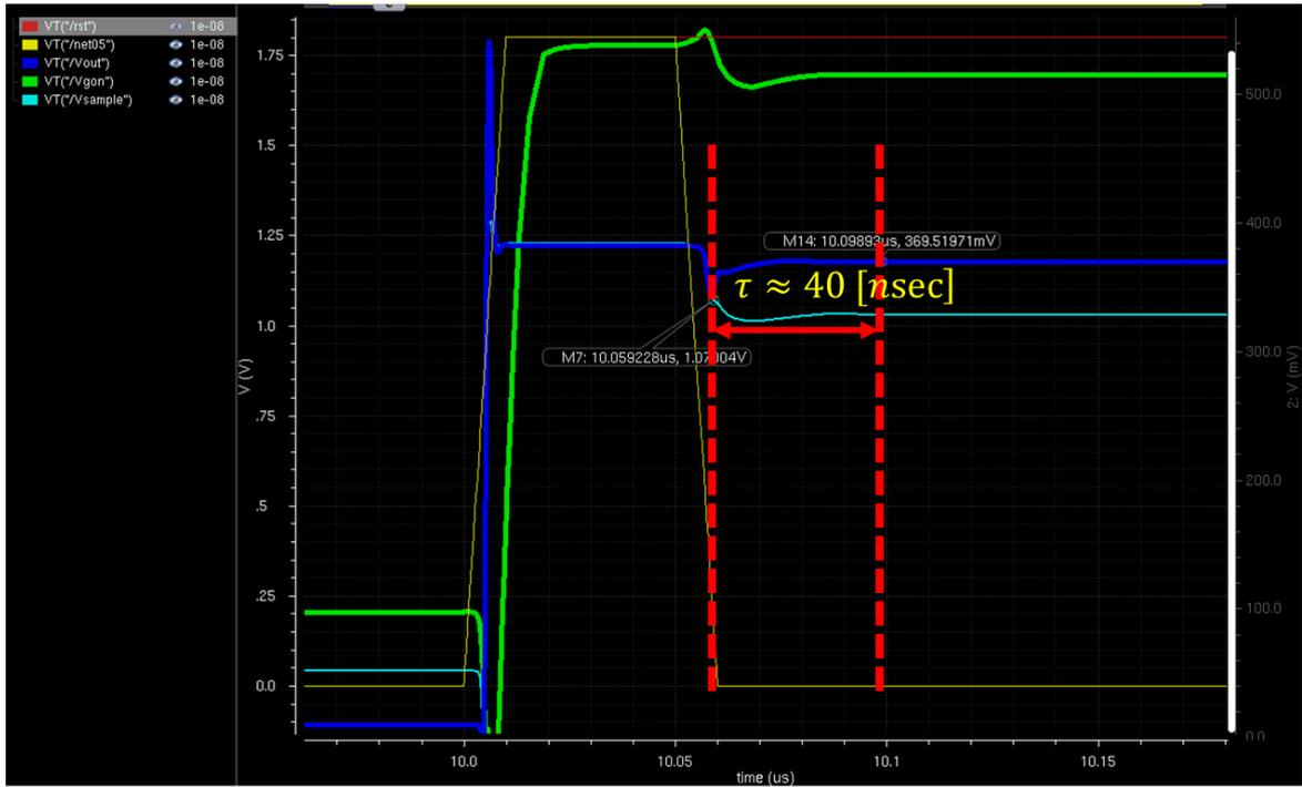
Figure 9: transient simulation results at 300K
