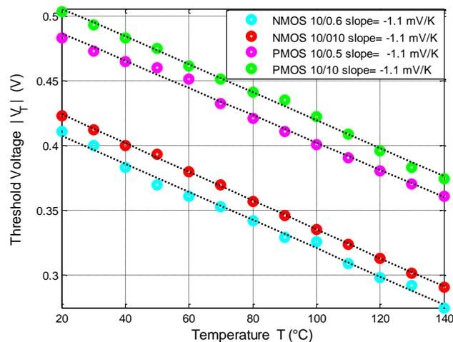
Figure 2 : Extracted threshold voltage of reference devices as a function of the chuck temperature
