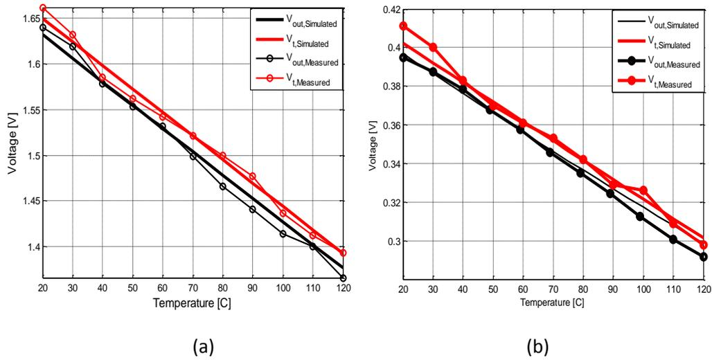
Figure 21: Measured and simulated output voltage of the  $V_t$  extractor circuit implemented in (a) CMOS-SOI 1 $\mu$ m process and in (b) CMOS 0.18 $\mu$ m process. The threshold voltage extracted during the thermal characterization process and the threshold voltage extracted from electrical Spice simulations are presented as well for both technologies.
