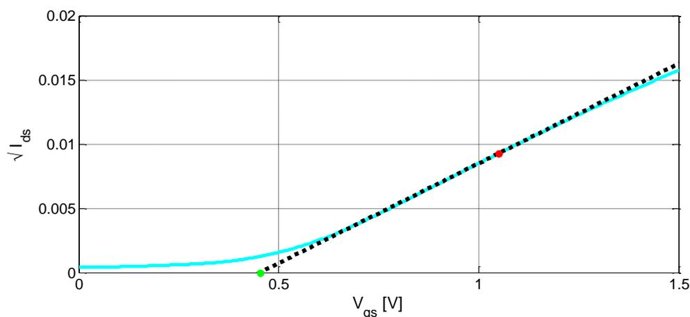
Figure 1: A graphical representation of the calculation procedure of the threshold voltage for the device shown in figure 2 at room temperature
