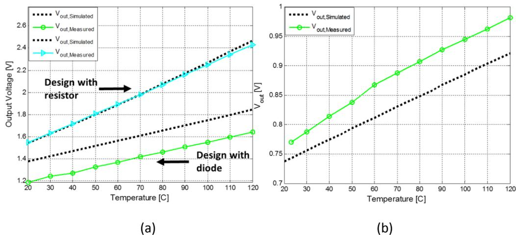
Figure 22: Measured and simulated output voltage of the PTAT circuits implemented in (a) CMOS-SOI 1 $\mu$ m process and in (b) CMOS 0.18 $\mu$ m process.
