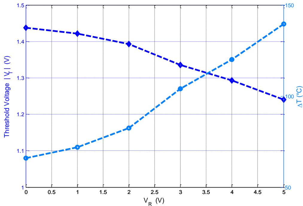
Figure 29: Extracted threshold voltage and the chip temperature rise determined from the process thermal characterization for different resistor voltages.
