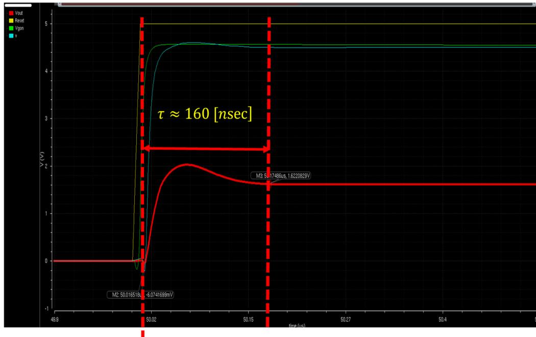
Figure 13: transient simulation results at 300K
