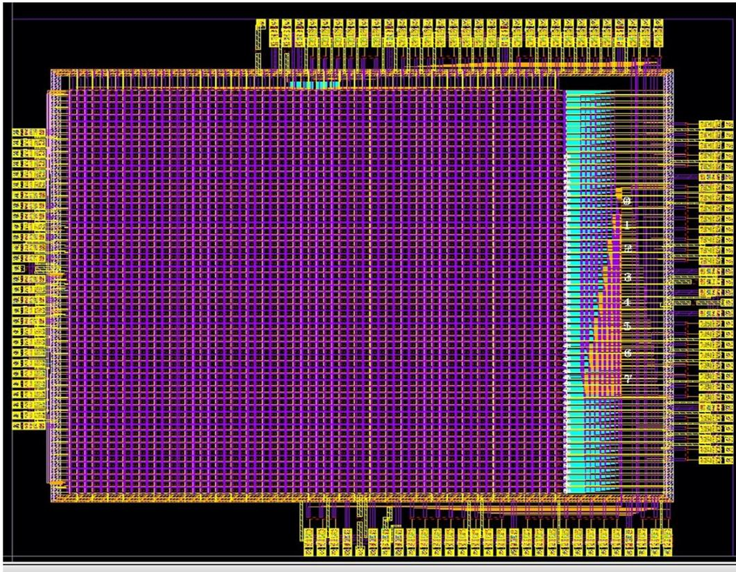
Figure 15: layout of 64 x 64 SPAD Array (top view)
