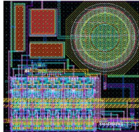
Figure 18: The SPAD structure, pixel structure and layout of the second design
