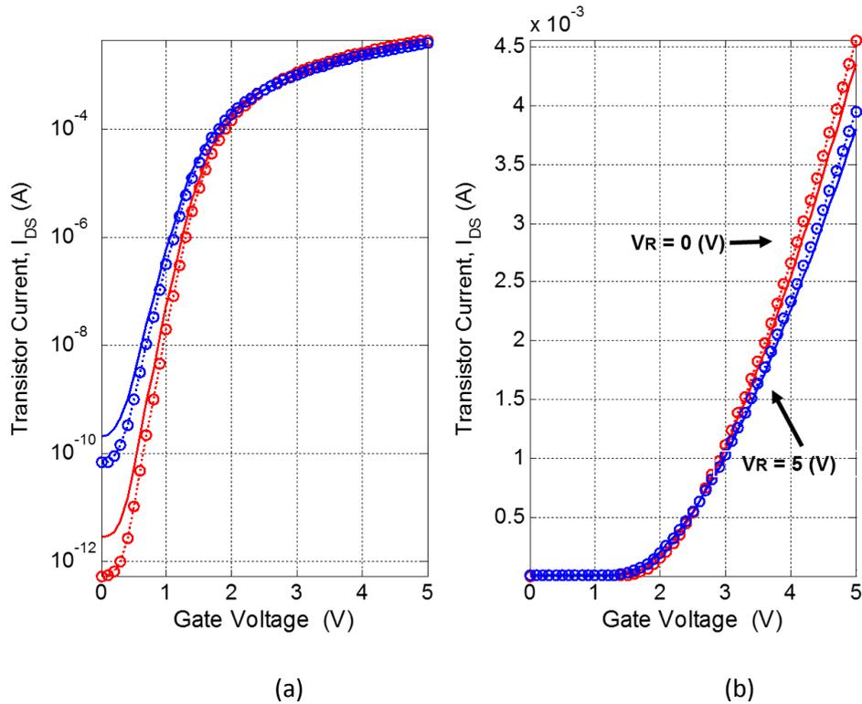
Figure 30: Example of I-V sweep performed while **cooling the chip** for an NMOS transistor with  $W/L = 178 \times 228 \mu\text{m} / 10.6 \mu\text{m}$ : on a semi-log scale (a) and on a linear scale (b). The dashed I-V curves were measured with cooling. The solid curves were measured without cooling.
