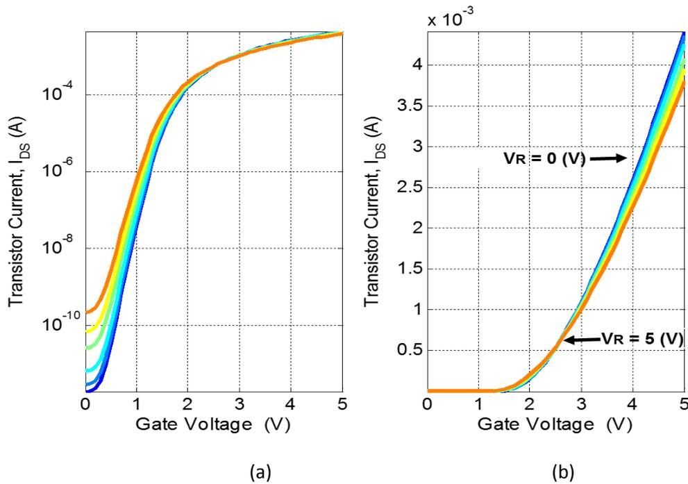
Figure 28: Example of I-V sweep performed for different resistor voltages for an NMOS transistor with  $W/L = 178 \times 228 \mu\text{m} / 10.6 \mu\text{m}$ : on a semi-log scale (a) and on a linear scale (b).
