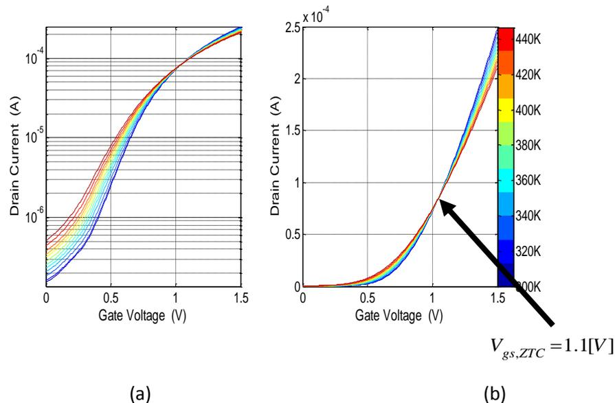
Figure 2: I-V sweep performed from room temperature till 440K on an NMOS transistor with  $W/L= 10 \mu\text{m} /0.6 \mu\text{m}$ : on a semi-log scale (a) and on a linear scale (b).
