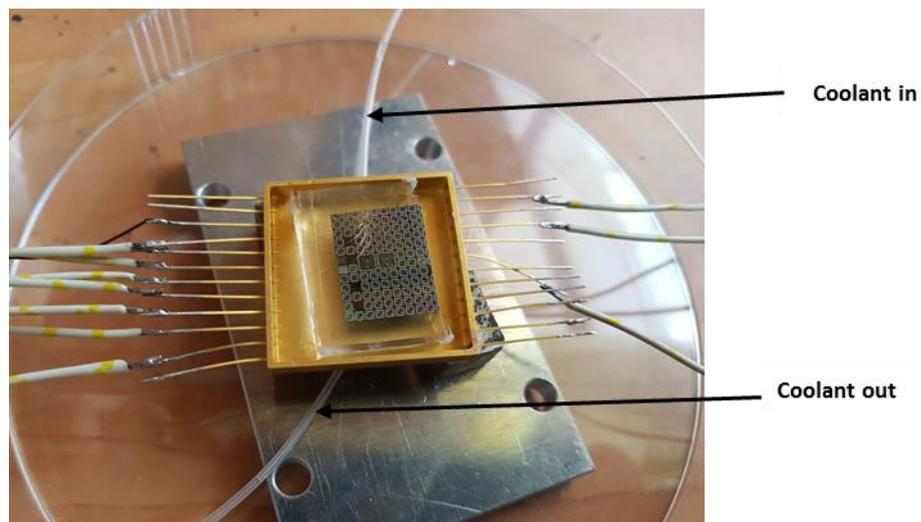
Figure 26: Packaging for electrical and thermal characterization
