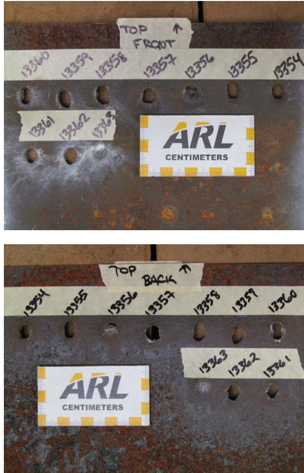
Fig. 15 Postballistic front and back side photographs of the 4.947-mm RHA plate vs. the 0.30-cal. M2 ball projectile. Note the lack of bulging for the penetrators that did not perforate the plate.
