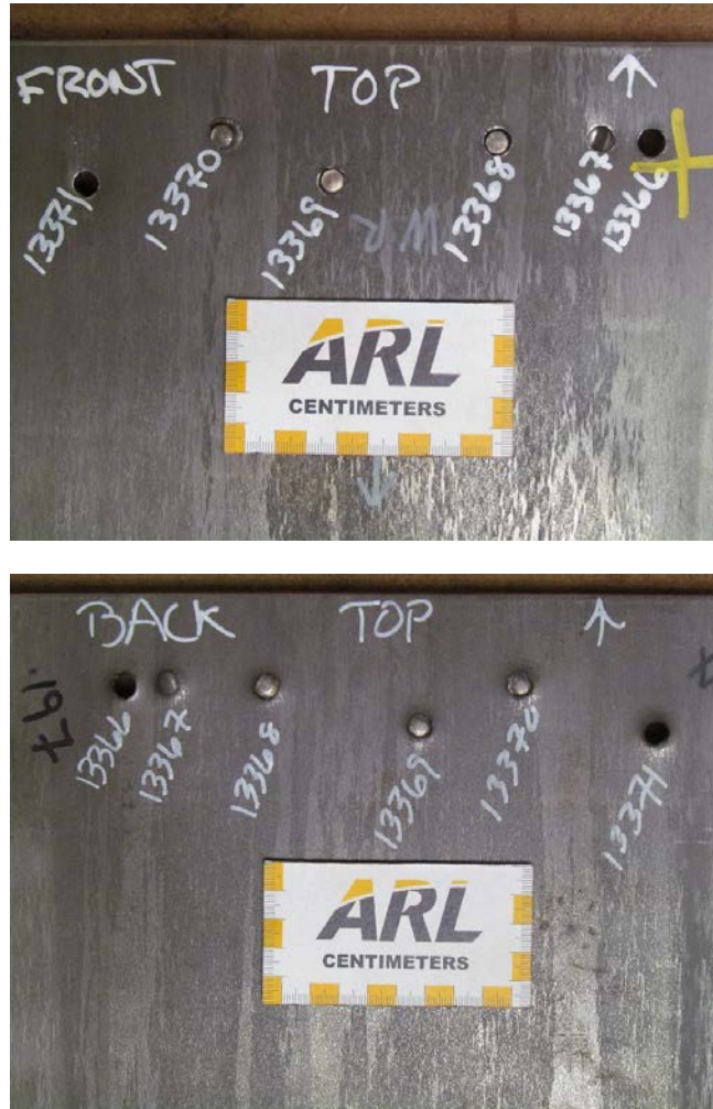
Fig. 16 Postballistic front and back side photographs of the 5.004-mm Salzitter steel plate vs. the 0.30-cal. FSP
