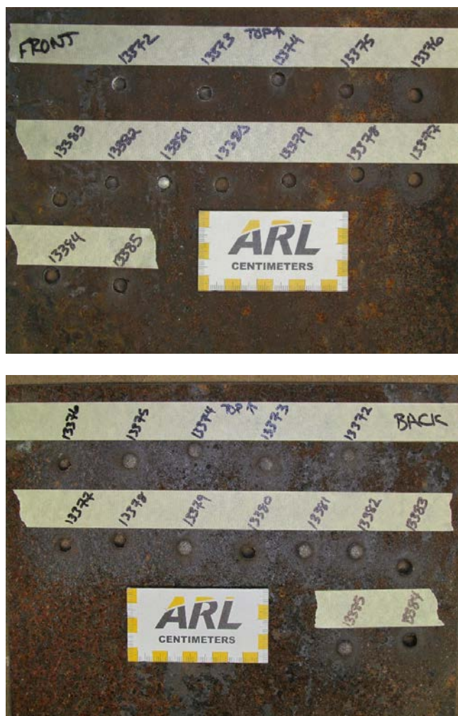
Fig. 17 Postballistic front and back side photographs of the 4.947-mm RHA plate vs. the 0.30-cal. FSP
