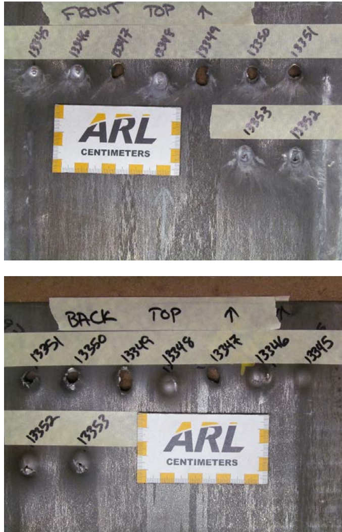
Fig. 14 Postballistic front and back side photographs of the 5.004-mm Salzgitter steel plate vs. the 0.30-cal. M2 ball projectile. Note the bulging of the back face for the penetrators that did not perforate the plate.
