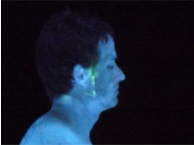
Figure 9. Black light photograph showing localized facial aerosol deposits after AST
