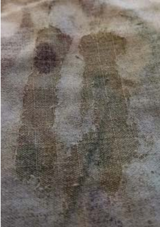
Figure 14. Configuration C4 (inner) after field wear from lower leg/boot abrasion
