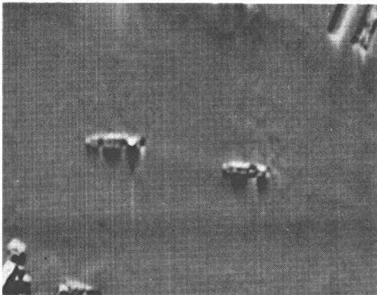
Fig. 21. A ship with one hot stack and a ship, apparently at anchor, with no hot stack. Date: 26 Jun 1962 Time: 2033 R Aircraft altitude: 2000 ft Air temperature (at 2000 ft): 82°F Water temperature: 78°F (estimated) Detector: Ge:Cu, 2.8 mm diameter Viewing angle: 6 degrees
