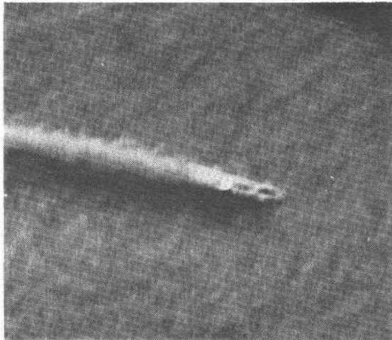
Fig. 12. Warm submarine on the surface. Date: 15 Mar 1962 Time: 2127 R Aircraft altitude: 1600 ft Air temperature (on surface): 79°F Water temperature: 74°F Detector: Ge:Cu, 2.8 mm diameter Submarine: USS GRENADIER (SS 525) Viewing angle: 30 degrees
