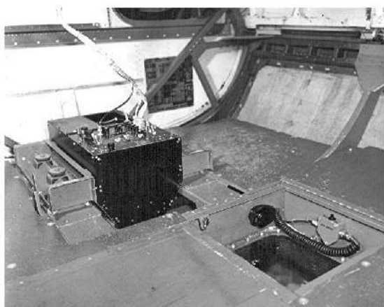
Fig. 1. AN/AAD-2 installed in modified bomb bay of SP-2E (P2V-5FS) aircraft.
