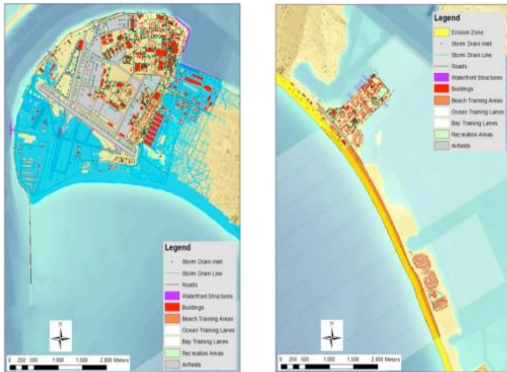
Figure 21. Left: flooding: Naval Air Station North Island (NASNI) – 1m sea level rise, 100-yr storm. Right: erosion: Naval Amphibious Base (NAB) – 1m sea level rise, 100-yr waves. (Based on work by Chadwick et al. (SERDP RC-1703).
