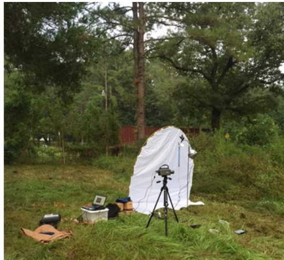
Figure 14. High-speed videography setup attempt at night collecting station.
