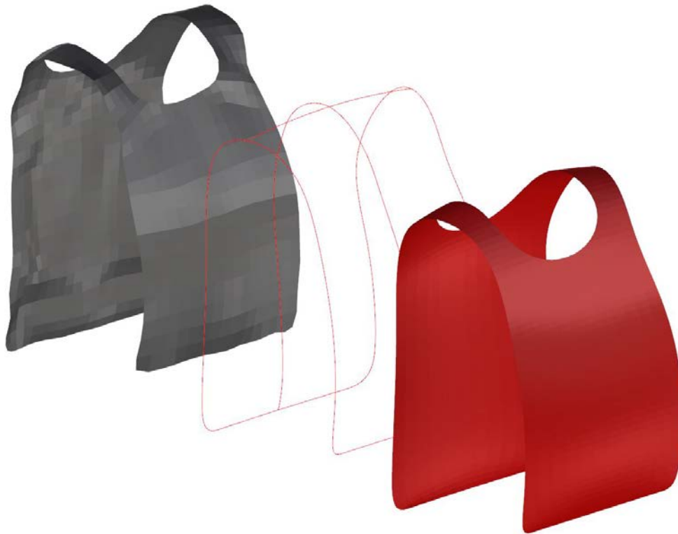
Fig. 5 The CT data for the SPS vest (gray, left) were used a guide to create curves representing the structure of the vest component (wire frame, center), and then the curves were used to develop the final idealized vest geometry (red, right) to be placed on ORCA man
