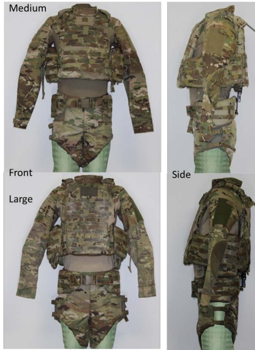
Fig. 9 SPS Tier 4 protection system shown on the foam ORCA body. The images provide a visual comparison of fit between the medium and large SPS systems on the foam ORCA manikin.
