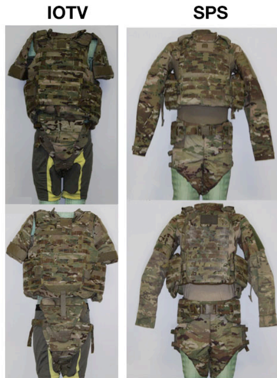
Fig. 1 Full IOTV (left) and SPS (right) systems on the foam ORCA manikin
