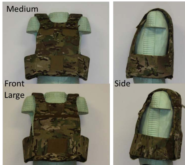
Fig. 8 SPS Tier 1 protection system shown on the foam ORCA manikin (without the shirt so that fit of vest could be better assessed). The images provide a visual comparison of fit between the medium and large SPS systems on the foam ORCA manikin.
