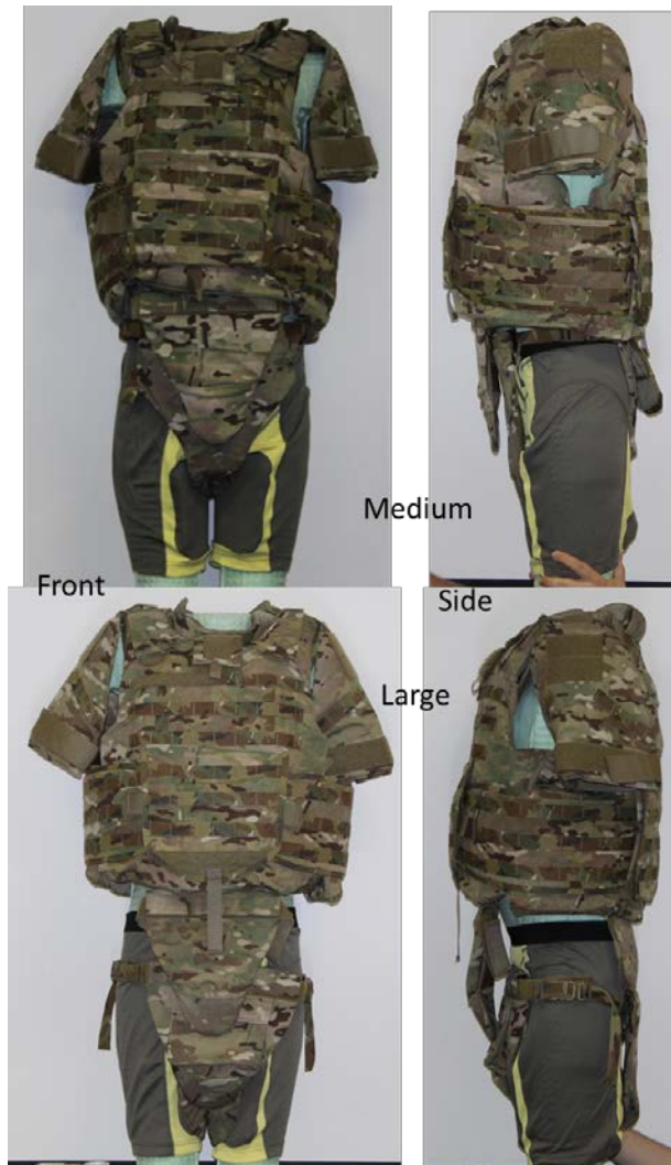
Fig. 10 IOTV protection system shown on the foam ORCA body. The images provide a visual comparison of fit between the medium and large IOTV systems on the foam ORCA manikin.
