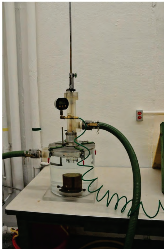
Figure 10. Specimen inside the chamber, ready for JET.
