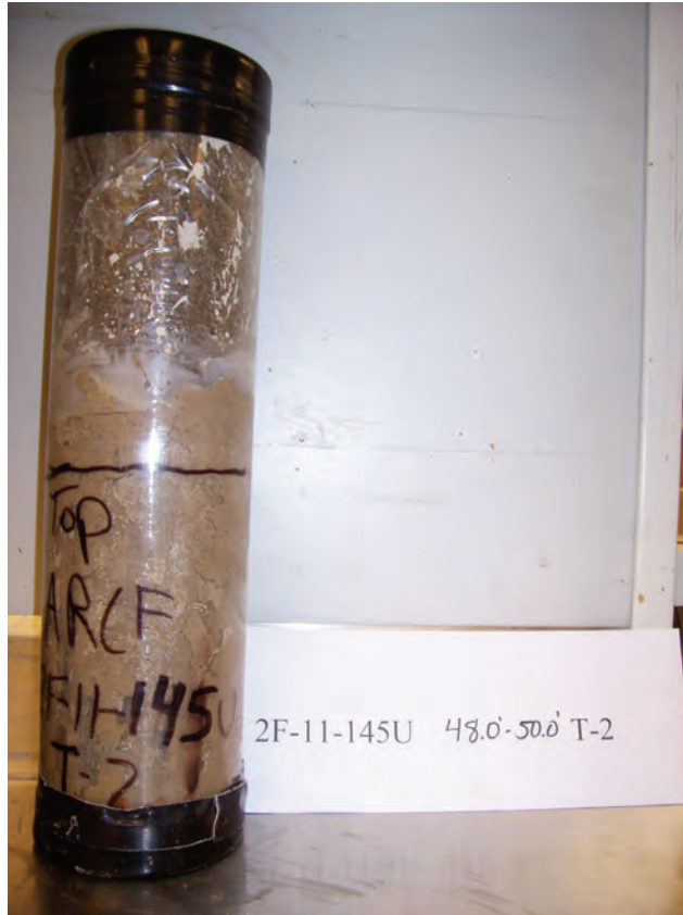
Figure B9. Sample from Boring 2F-11-145U Tube 2 with depth of 48.0 to 50.0 ft.
