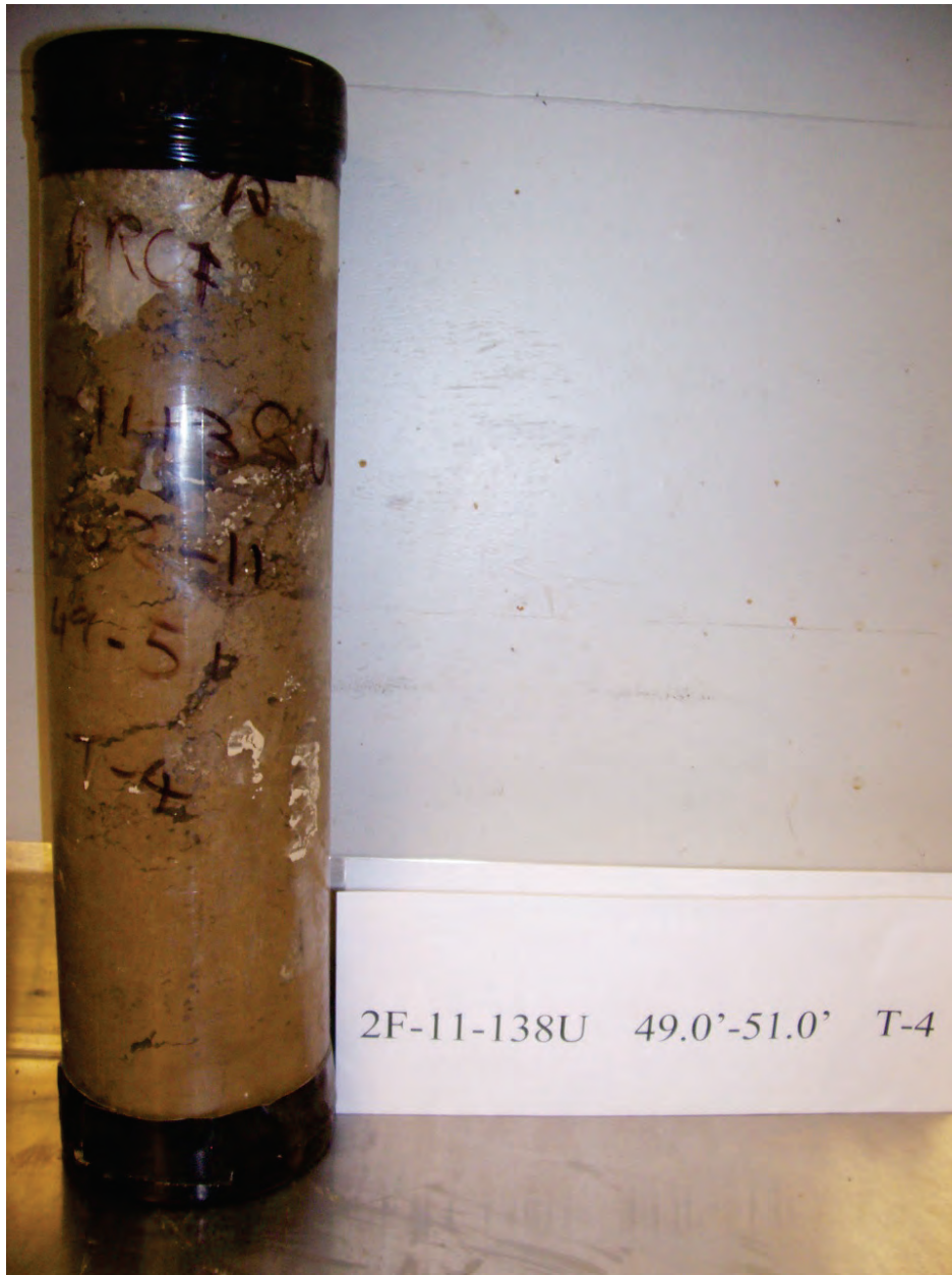
Figure B2. Sample from Boring 2F-11-138U Tube 4 with depth of 49.0 to 51.0 ft.
