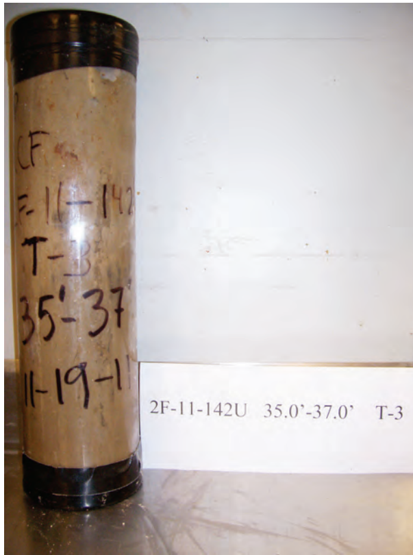
Figure B6. Sample from Boring 2F-11-142U Tube 3 with depth of 35.0 to 37.0 ft.
