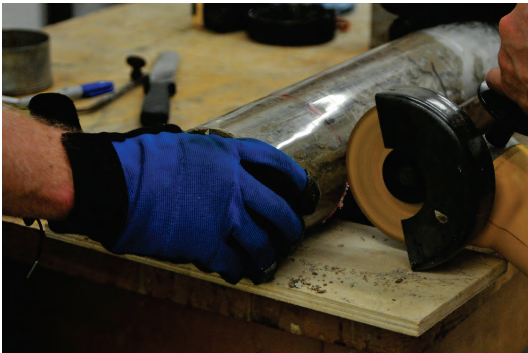
Figure 8. Using grinder to cut Plexiglas tube.
