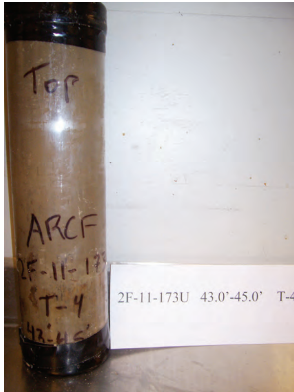
Figure B16. Sample from Boring 2F-11-173U Tube 4 with depth of 43.0 to 45.0 ft.
