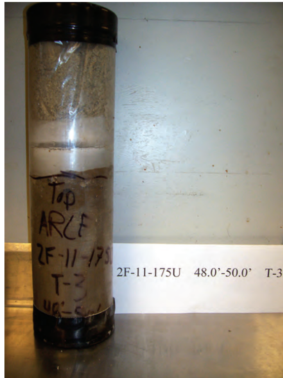
Figure B20. Sample from Boring 2F-11-175U Tube-3 with depth of 48.0 to 50.0 ft.
