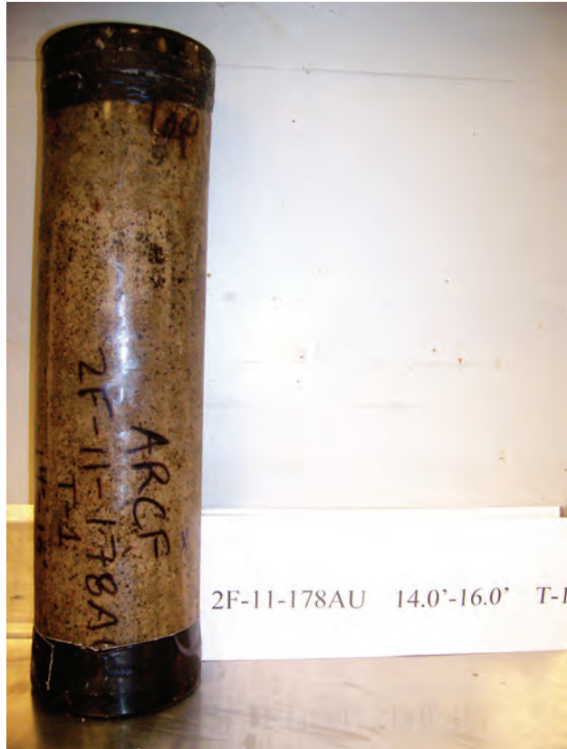
Figure B22. Sample from Boring 2F-11-178U Tube-1 with depth of 14.0 to 16.0 ft.
