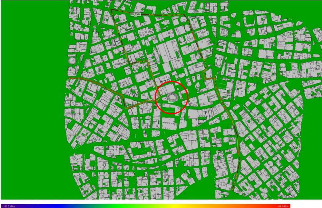
Figure 10. VANE urban scene model of a single Tx (Tx 3) atop a 332 m tall, centrally located high-rise building. Propagation paths are shown to an arbitrary Rx route through the city.
