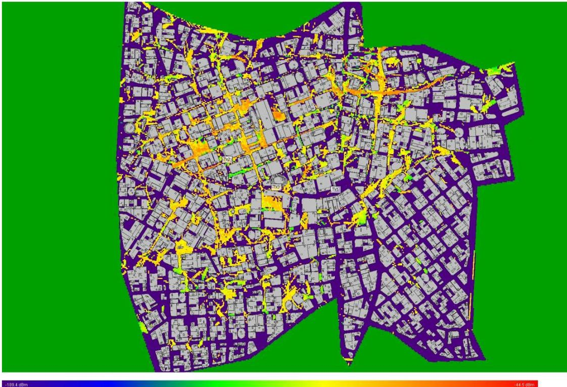
To conclude this section, note how signal power is channeled along low-lying, continuous urban canyons, much like a waveguide, in Figure 11 and Figure 12. This phenomenon is unique to dense urban zones and essential to consider in robotics telemetry scenarios when the base station and robot are along a line-of-sight or NLOS urban canyon (Li et al. 2012).
