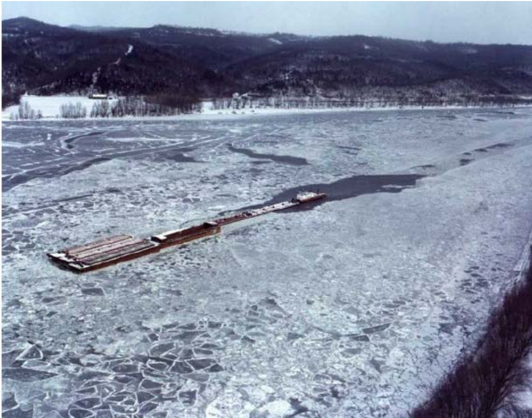
Figure 5. A tow breaking through brash ice on the Ohio River (Tuthill et al. 2004).
