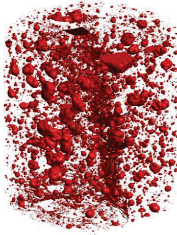
Figure 3. XMT image reconstruction showing voids within a damaged specimen (Oesch 2015).
