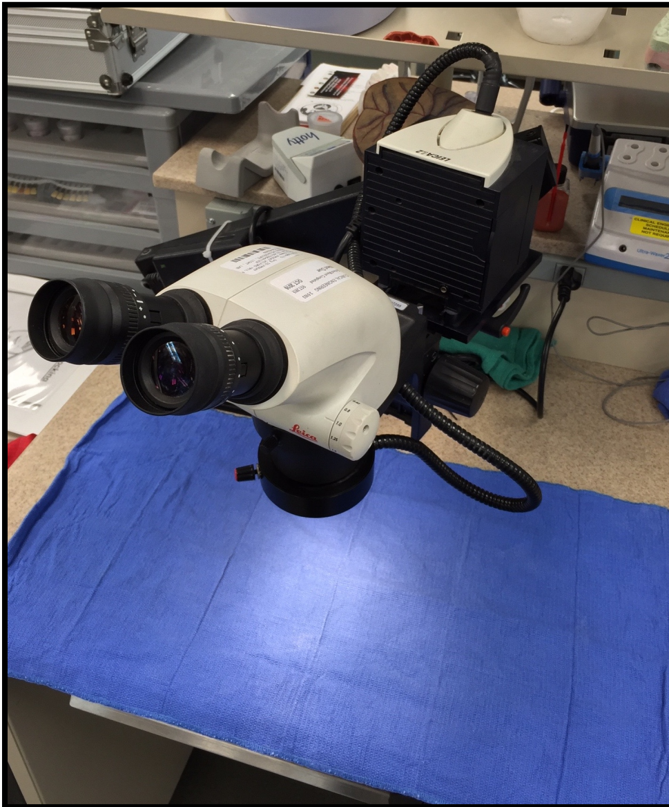
Figure 21: Leica S4 E Stereo Microscope for ARI Survey
