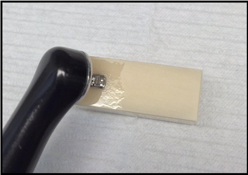
Figure 16: Bracket Light-Cured from All Four Sides
