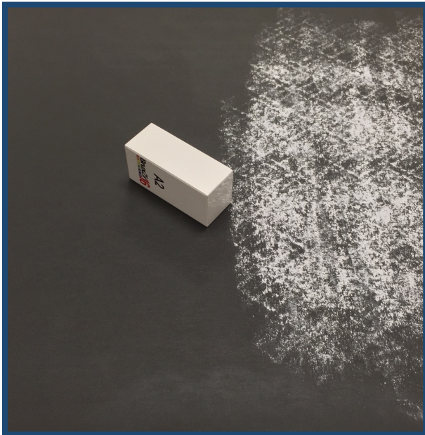
Figure 4: Sanding of the Sample Surfaces with 600-Grit Silicon Carbide Paper
