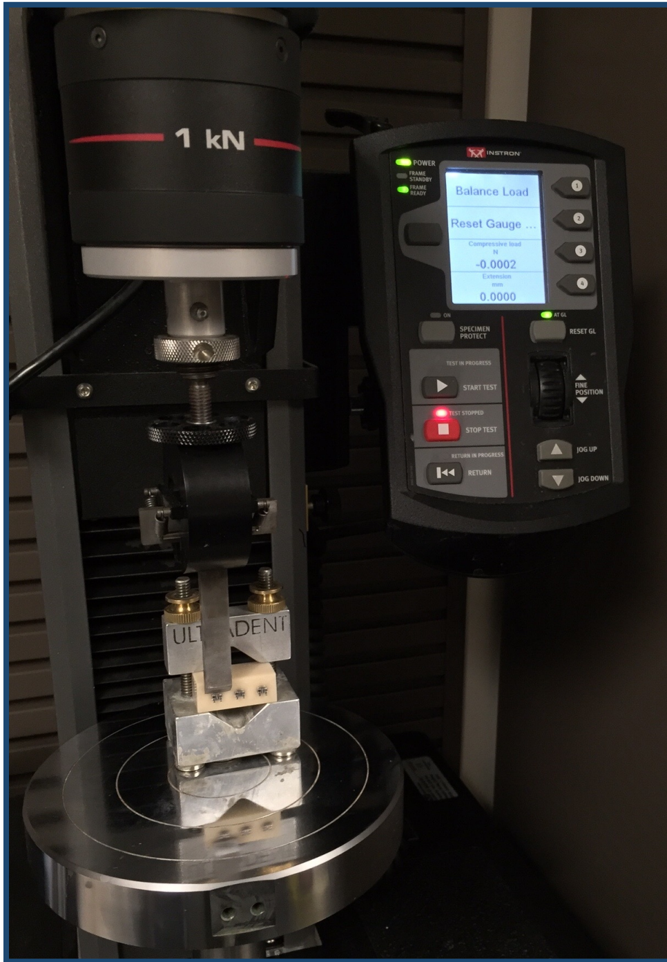
Figure 18: Mounted Substrate Blocks on Jig
